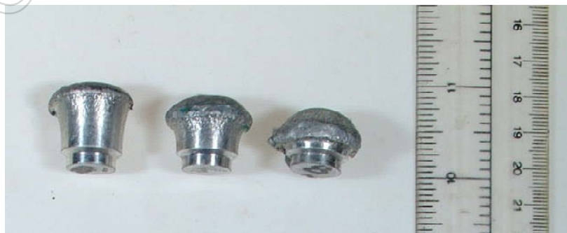
Deformed aluminum projectiles after plate perforation.
