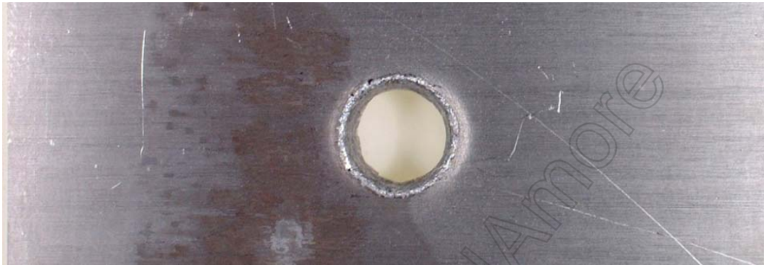
Perforated 0.5 in (12.7 mm) aluminum plate.
