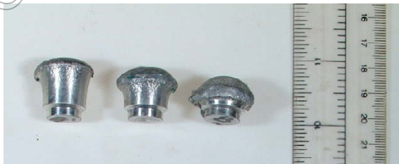
Deformed aluminum projectiles after plate perforation.
