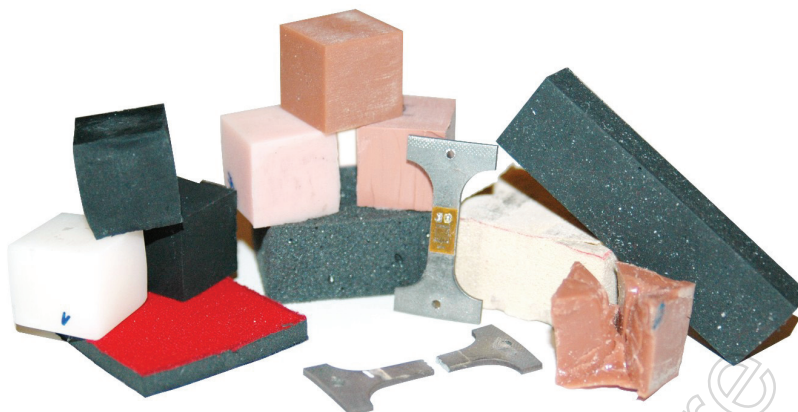
Figure 10: Material test samples of the WorldSID
