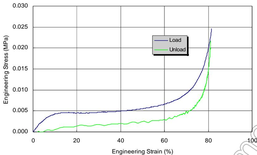
Figure 4 Load-recovery data for a polyurethane foam
