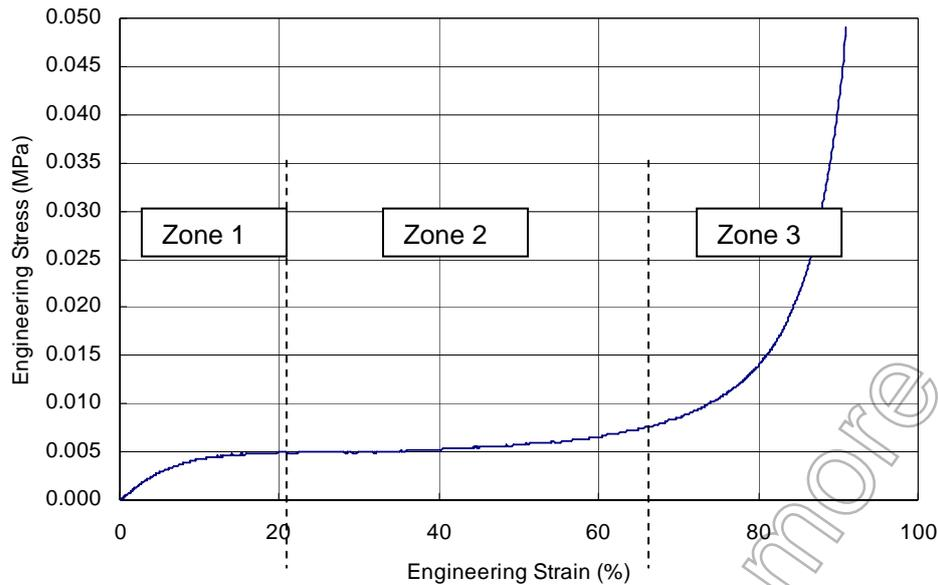
Figure 1 Three deformation zones typically observed in foams
