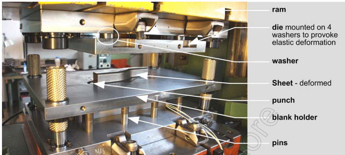
Figure 6: Tool set-up for experimental evaluation of die surface compensation
