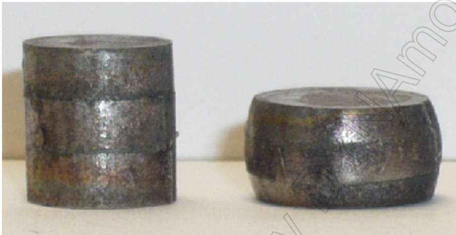
Figure 6: Undeformed and deformed specimen.
