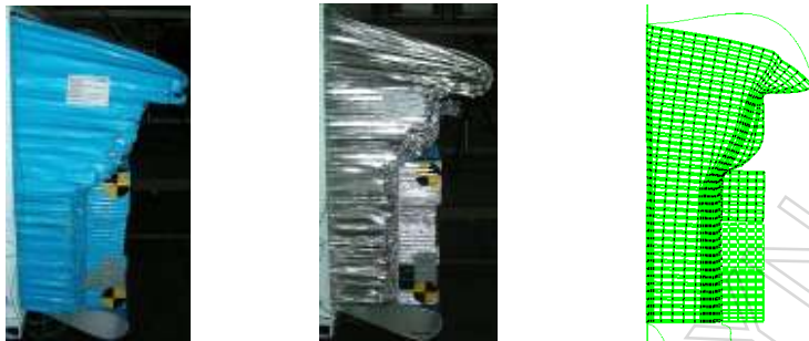
Figure 11: Deformed barriers test 1, 2 and simulation;
