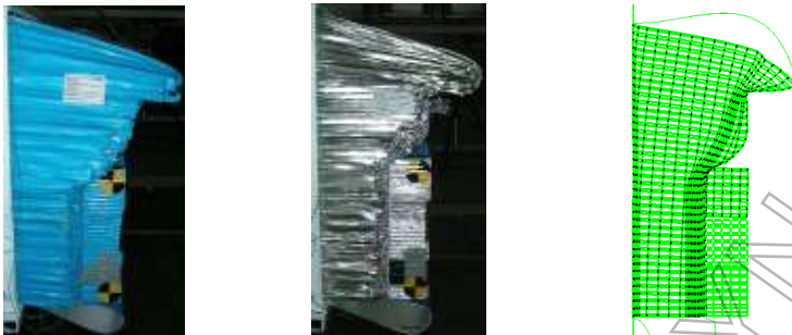
Figure 11: Deformed barriers test 1, 2 and simulation;
