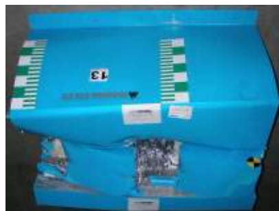
Figure 17: Deformed barriers test 13 and simulation;
