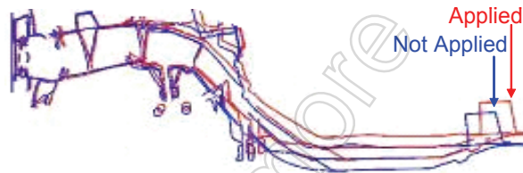
Fig.9 Side member deformation([1]Frontal impact)
