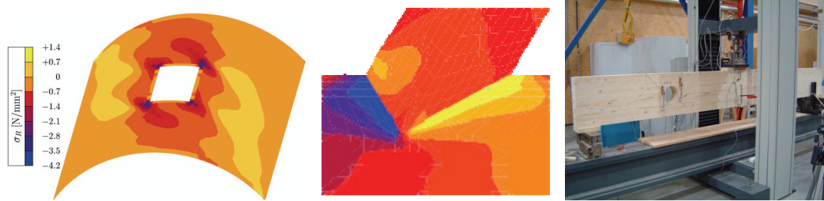
Figure 11: Experimental investigation and FE analyses of wooden structures (a) distribution of stress component perpendicular to the fiber direction, (b) distribution of in-plane component of shear stresses, and (c) experimental set-up of structural test [15], [16]
