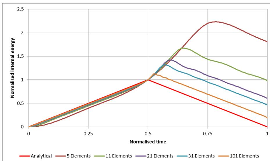
Fig. 7: Normalised internal energy of strain-softening bar for  $0 \leq t \leq 2 \cdot L/c_e$
