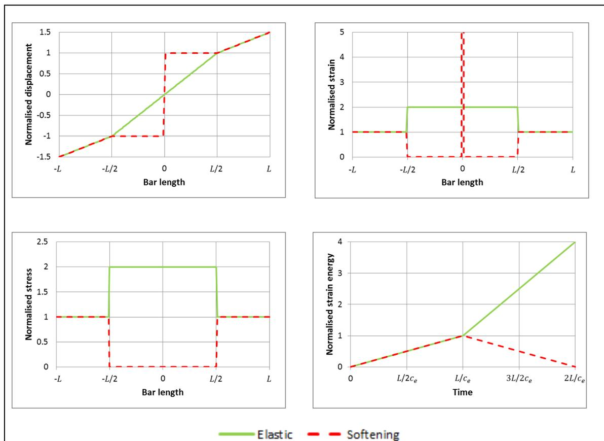
Fig. 3: Analytical solution for displacement, strain and stress for  $t = 3/2 \cdot L/c_e$  and internal energy over time
