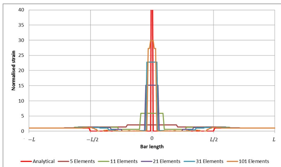
Fig. 5: Normalised longitudinal strain of strain-softening bar at  $t = 3/2 \cdot L / c_e$
