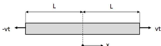
Fig. 2: Geometry and loading of strain-softening bar [2]
