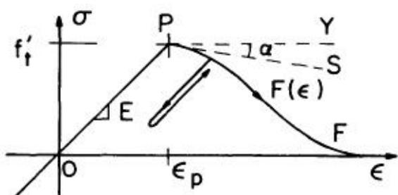
Fig. 1: Stress-strain diagram of strain-softening material [2]
