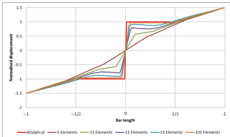
Fig. 4: Normalised longitudinal displacement of strain-softening bar at  $t = 3/2 \cdot L / c_e$
