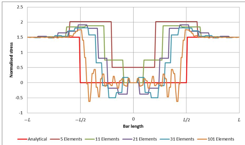
Fig. 6: Normalised longitudinal stress of strain-softening bar at  $t = 3/2 \cdot L/c_e$
