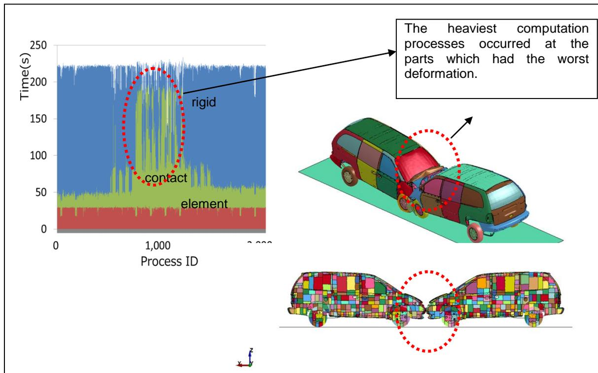
Fig3. all ranks timing costs (left) , deformed parts(right above) and decomposition image(right below) by 2048 process
