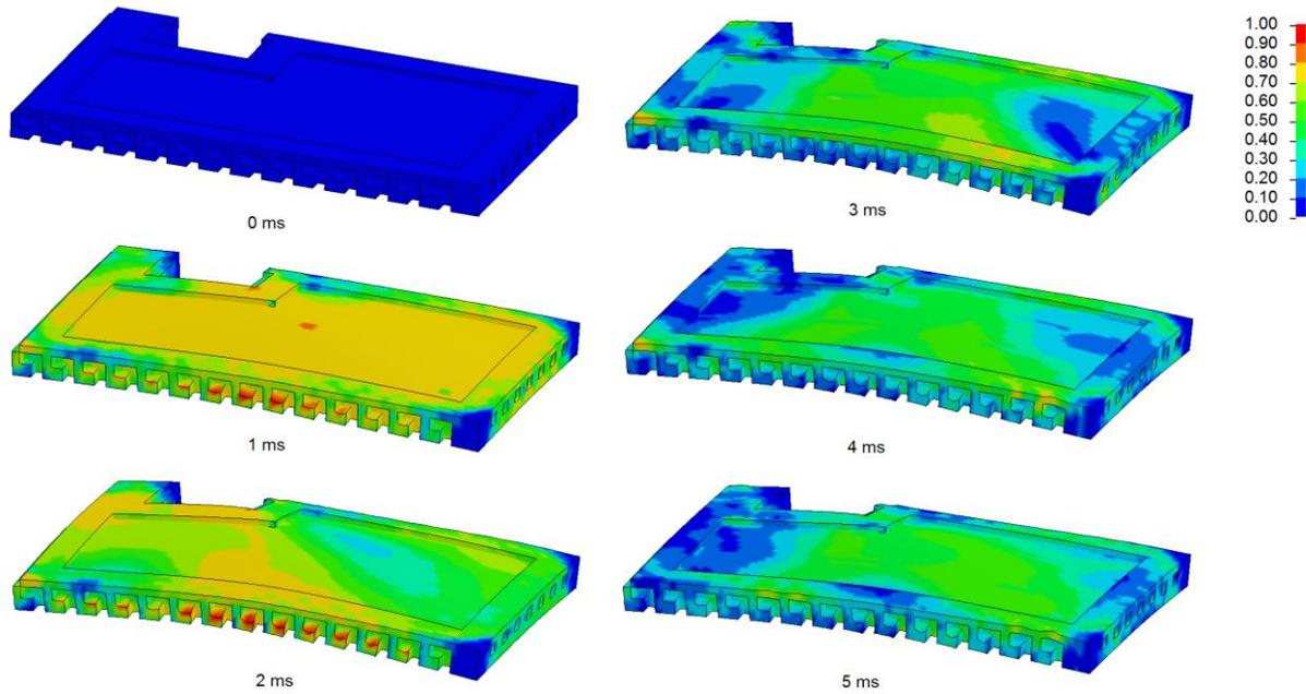
Fig. 9: Normalized Von-Mises stresses (Concept 3)
