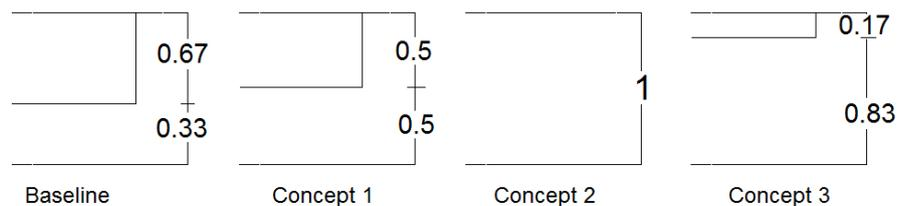
Fig. 4: Comparison of the relative thicknesses of the protection plate a) Baseline (waffle cross-section) b) Concept 1 (waffle cross-section) c) Concept 2 (full plate) d) Concept 3
