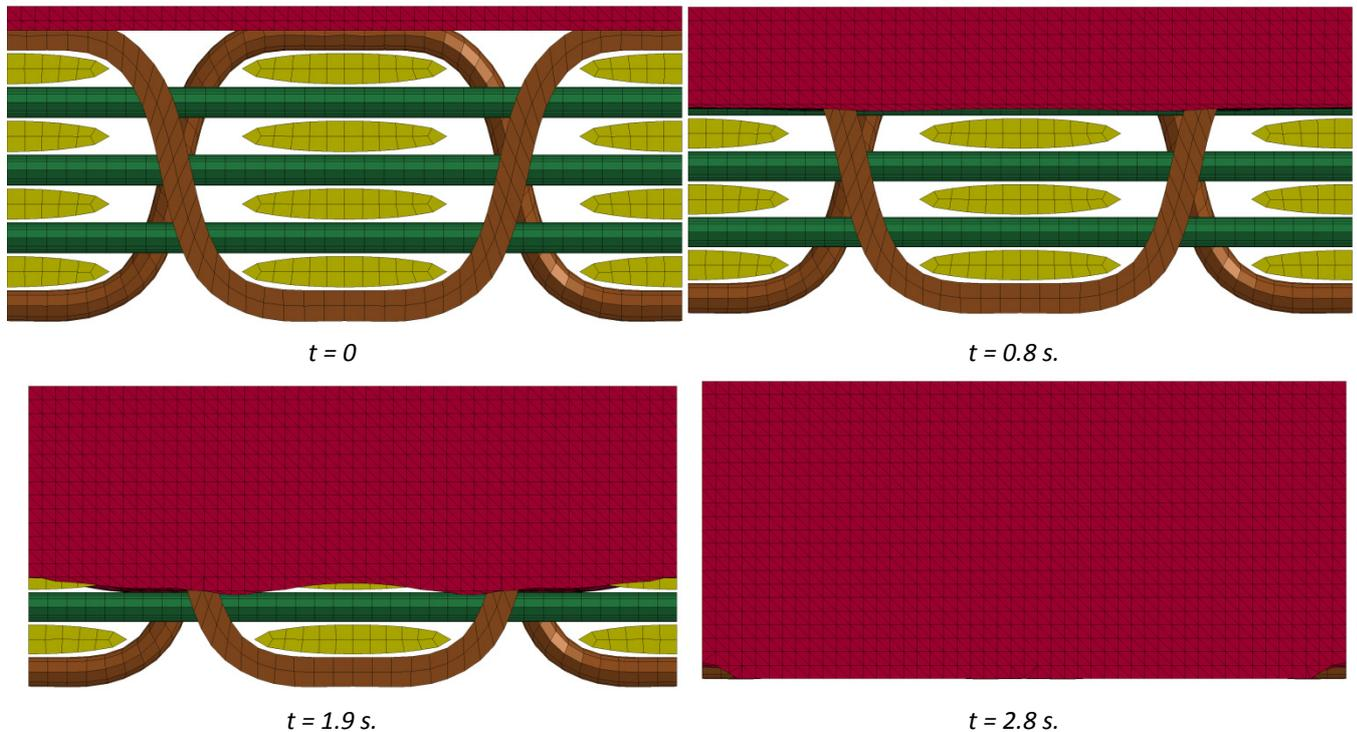
Fig. 6: Resin flow through the RVC.
