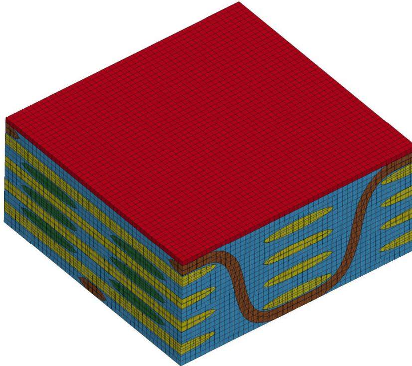
Fig. 4: FE model for RTM modeling in stitch direction.
