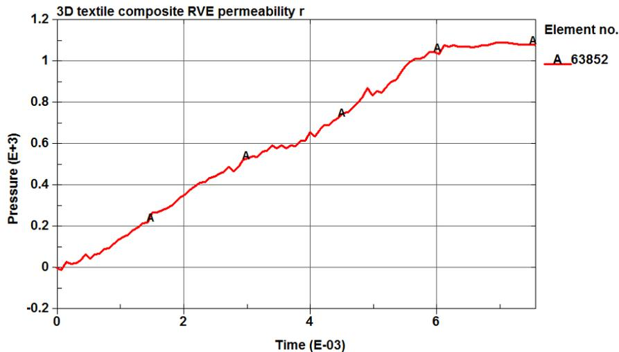
Fig. 7: Pressure drop chart in Y-direction, Pa.
