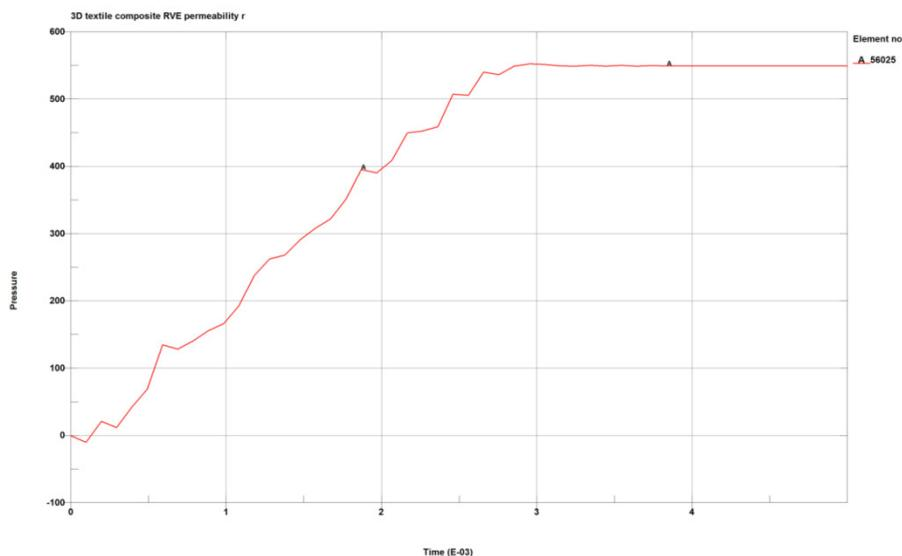
Fig. 5: Pressure-time chart for resin flow in Z-direction. Time scale is 1/1000. Pressure is in Pa.
