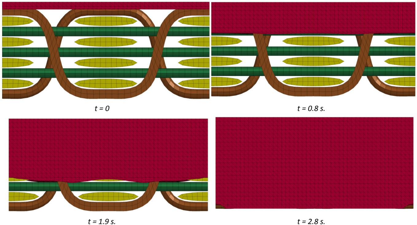
Fig. 6: Resin flow through the RVC.
