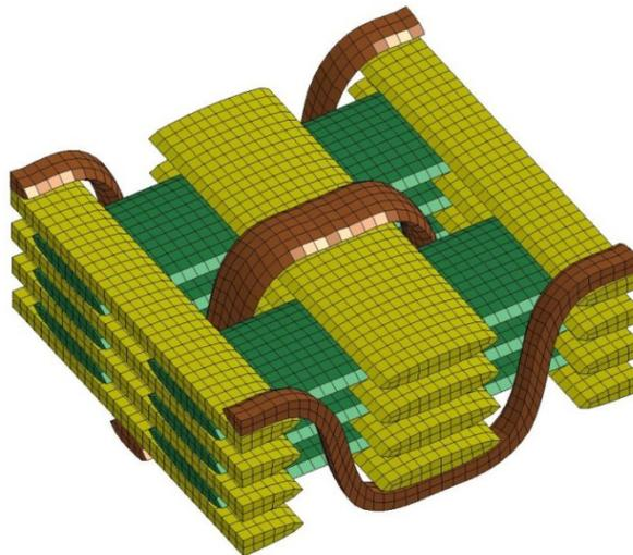
Fig. 3: Finite element model of the RVC.
