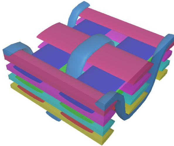
Fig. 2: The RVC geometry in TexGen.
