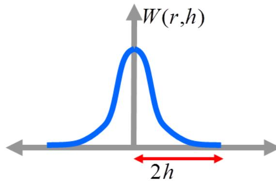
Fig 1. Support size of 2d kernel function
