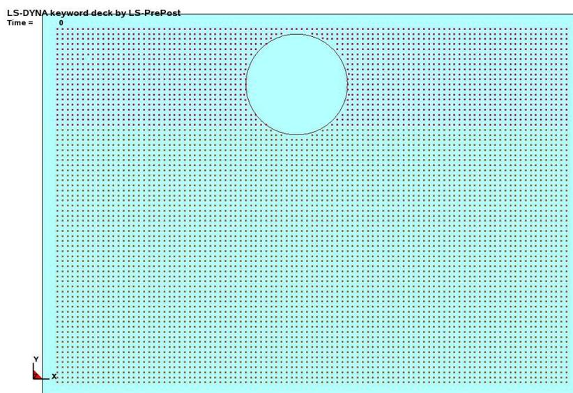
Fig 7. Problem set up of water impact
