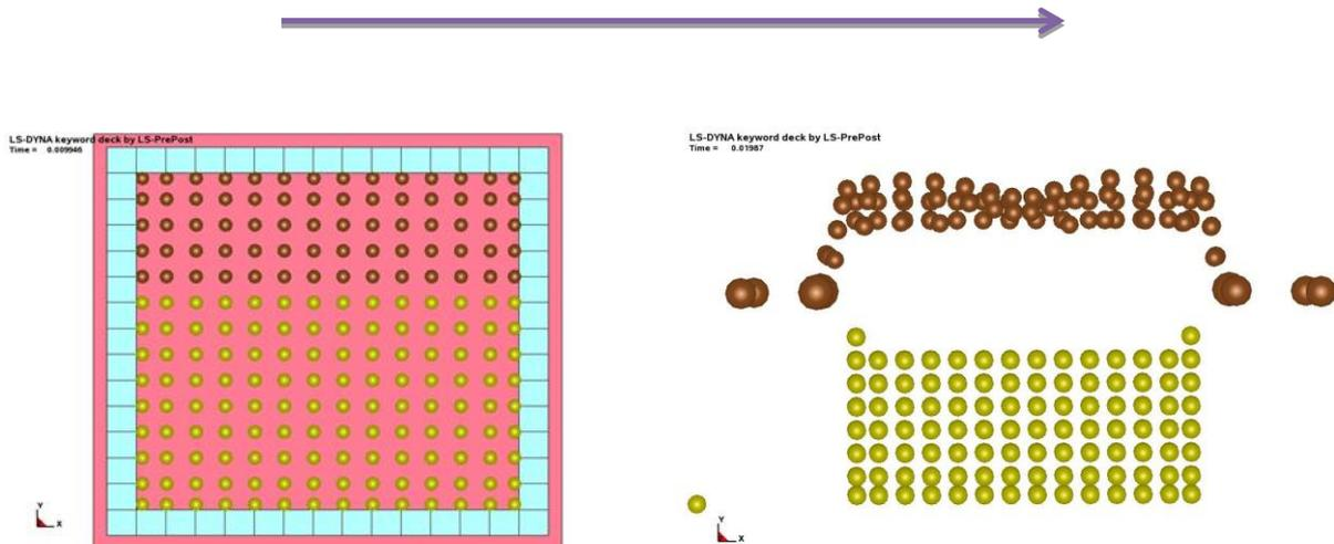
Fig 3. Instability on the interface for tank sloshing with SPH interpolation method
