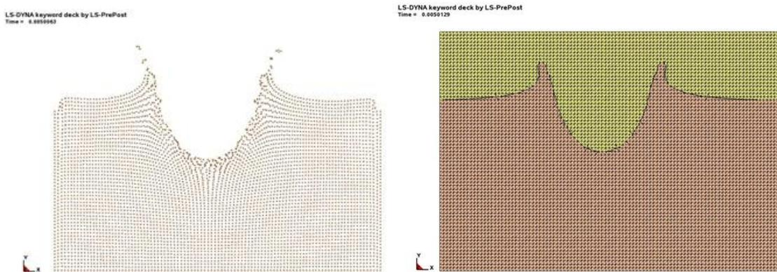
Fig 9. Final deformation shape from SPH model (left) compared to ALE model (right)
