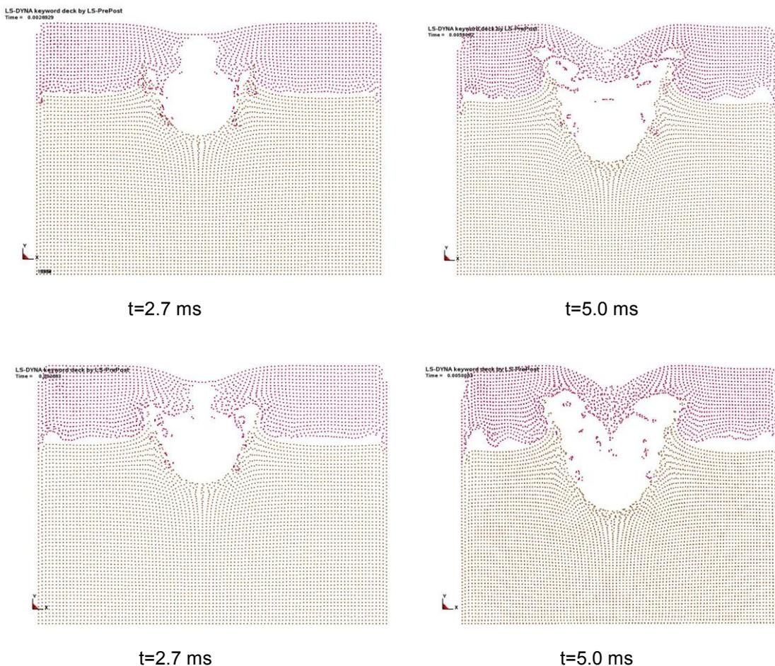
Fig 8. Upper: deformation shape for air and water model
