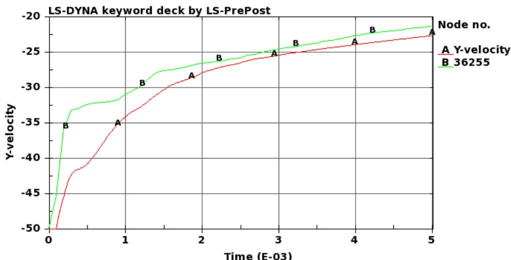
Fig 10. Impact velocity from SPH model (B) compared to velocity from ALE model (A)
