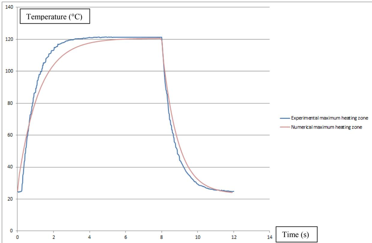
Figure 10 Heating and cooling. Temperature behavior: comparison between experimental point p1 and equivalent numerical location
