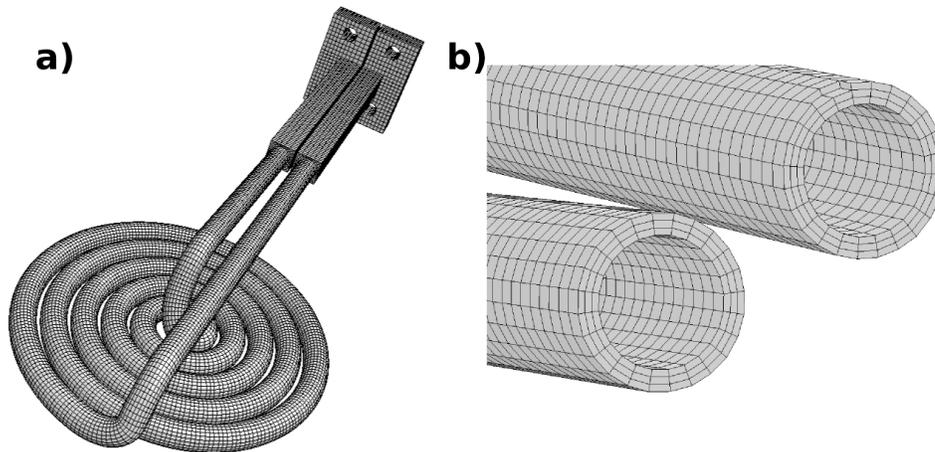
Figure 5 Coil geometry and mesh. a) Global view, b) Zoom on inner section
