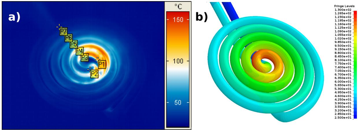
Figure 9 Comparison for coil temperature between a) Experimental results from thermal camera, b) Numerical simulation results
