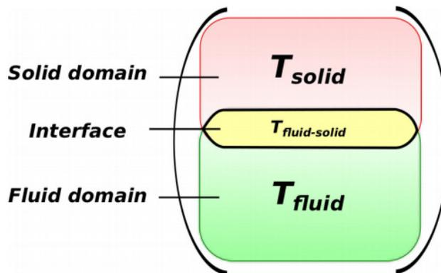
Figure 2 Vector of temperature unknowns when the fluid thermal solver and structure thermal solvers are coupled using a monolithically approach.
