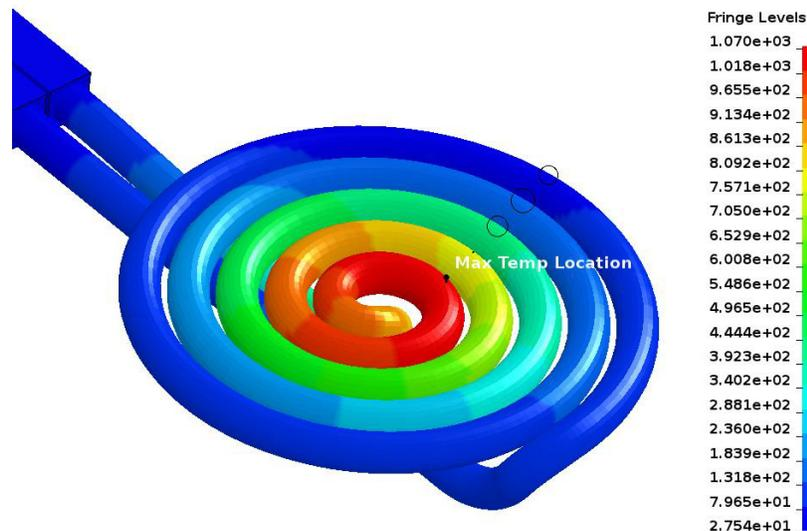
Figure 6 EM-thermal only maximum temperature increase after 15 seconds at 394.85 A
