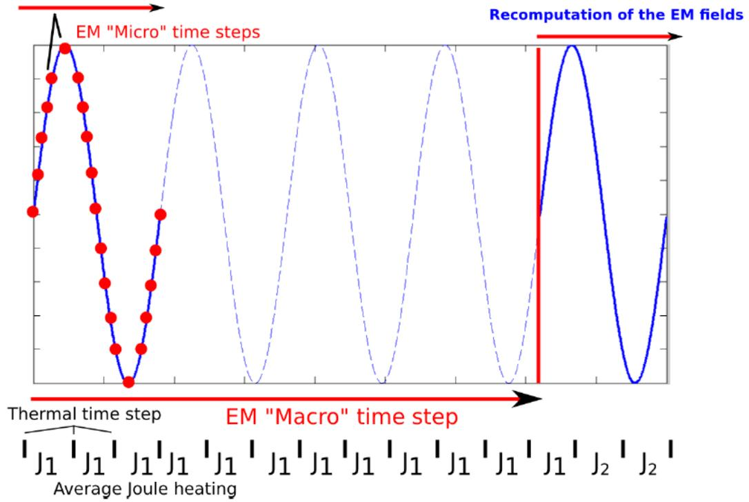
Figure 1 Graphical representation of the electromagnetic field and resulting joule heating calculation scheme implemented in the LS-DYNA inductive heating solver
