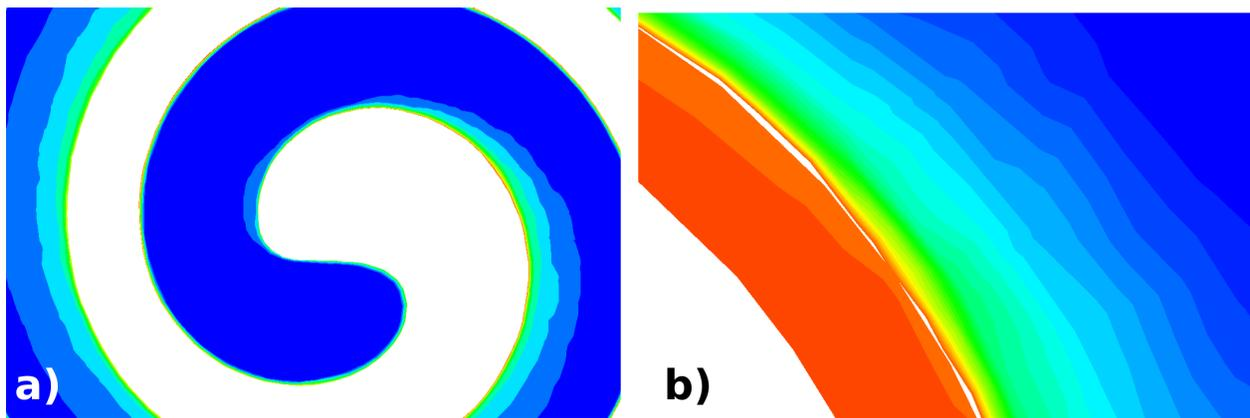
Figure 8 Temperature fringes : a) Fluid only, zoom on central part. b) Fluid and structure zoom on coil section
