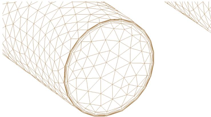
Figure 7 Fluid mesh: zoom on the inflow section
