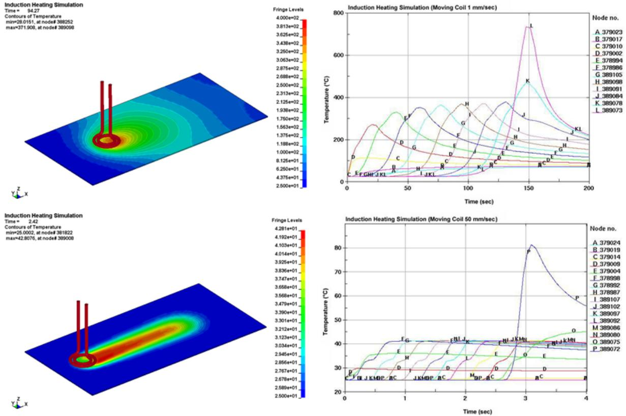
Figure 4 Graphical representation of the electromagnetic field and resulting joule heating calculation scheme implemented in the LS-DYNA inductive heating solver
