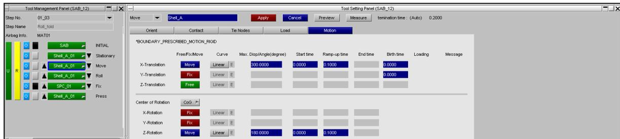
Fig. 4: Motion setting for move type tool mesh in TSP
