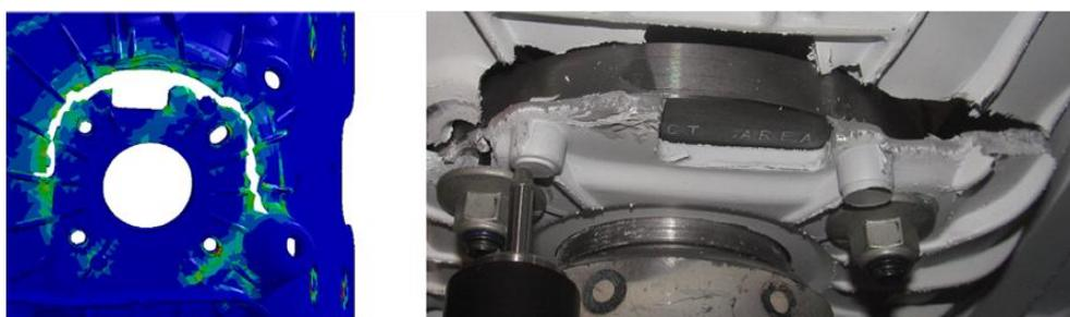
Fig. 15: Crack propagation in tetrahedron finite element model and real shocktower
