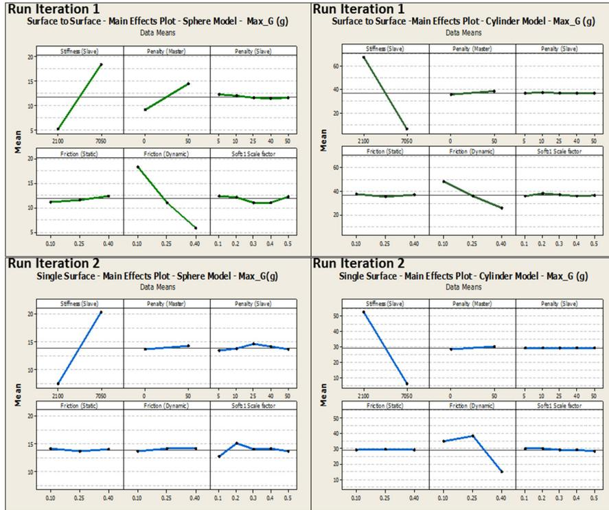
Figure 7: Sphere & Cylinder Main Effects plot (Surface to Surface, Single Surface & Single Surface Enhanced)
