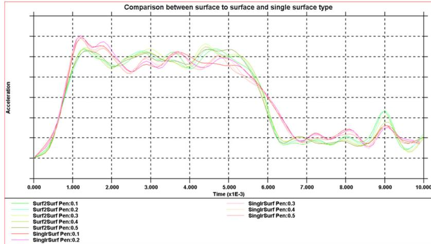
Fig. 9: Comparison between Surface to Surface and Single Surface Type Vs Penalty factor - Cylinder to Dome
