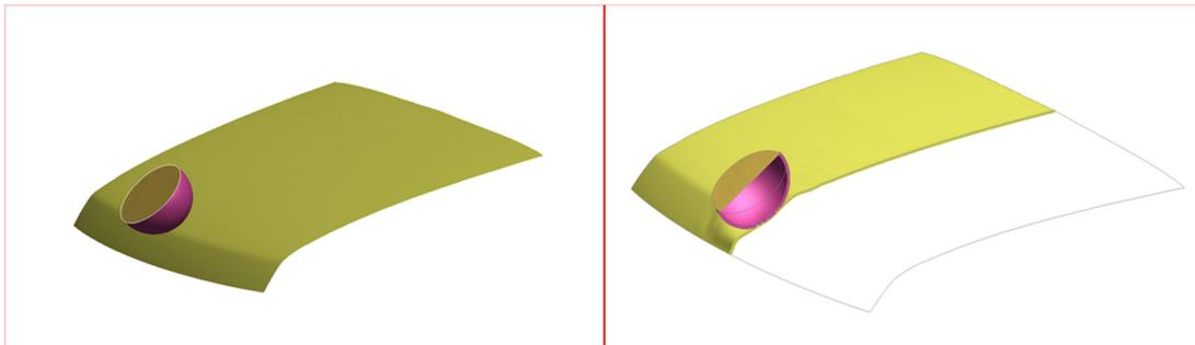
Fig. 3: Sphere Model Impacting a Dome
