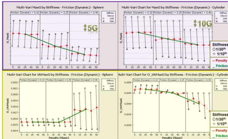
Fig.5: Multivariability Study by Stiffness – Sphere Model
