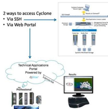
Fig. 4: SGI Cyclone – HPC on-demand Cloud Computing
