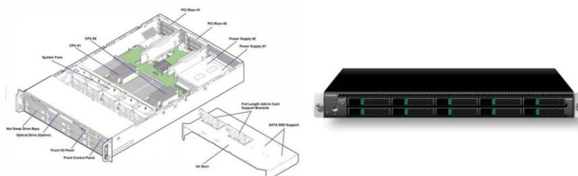
Fig. 1: Overhead View of SGI Rackable Server with the Top Cover Removed and Actual Server
