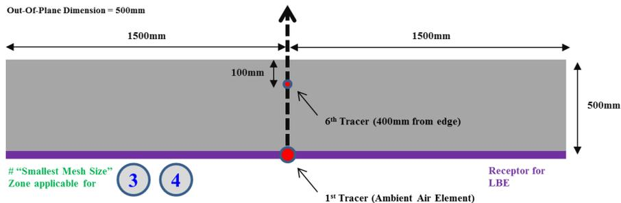
**Figure 3: Location of Tracers & Smallest Mesh Size Zone (LBE MM-ALE)**
