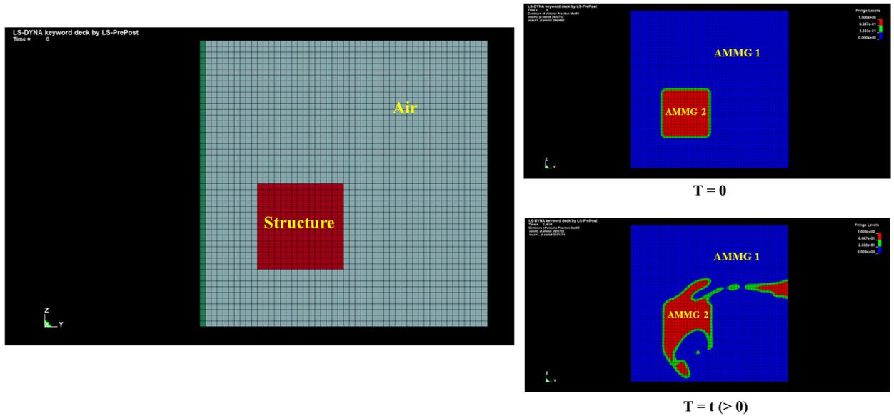
Figure 5: Illustration of Leakage (Couple to “Air Outside” only)
