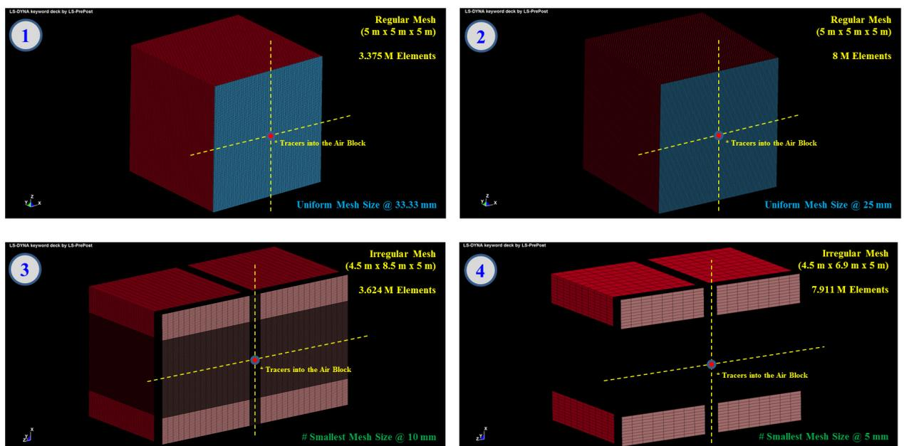
Figure 2: Four Air Configurations considered (LBE MM-ALE)
