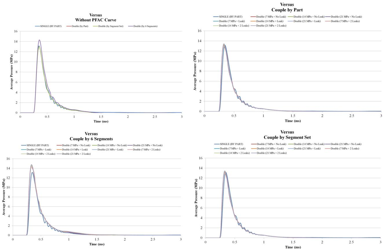
Figure 7: Average Coupling Pressure of Front Segment for All Cases
