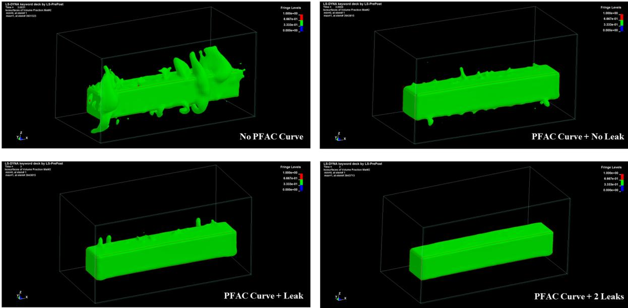
Figure 6: Typical Volume Fraction Plots of the Four Combinations
