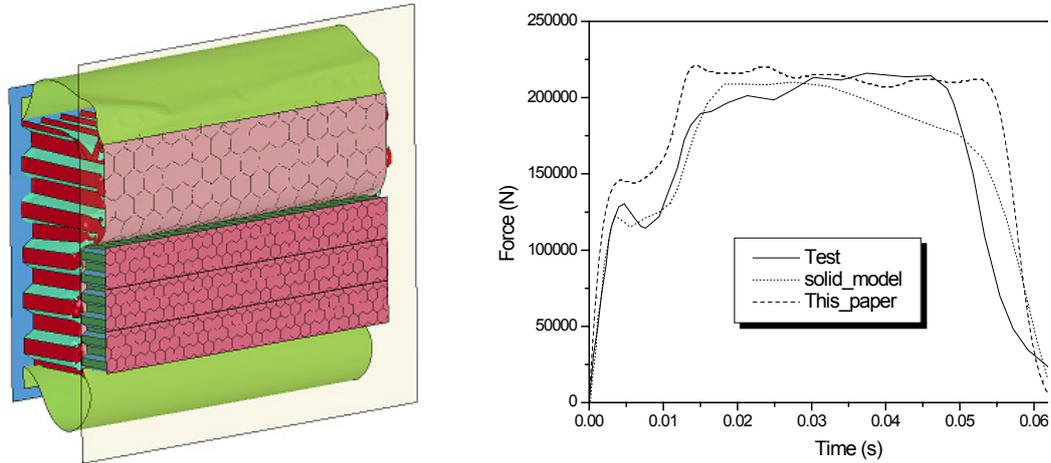
Fig. 8: Results of ODB impacted with flat wall
