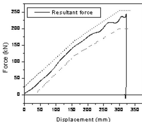
Fig. 4: Resultant force of MDB in dynamic test of ECE R95
