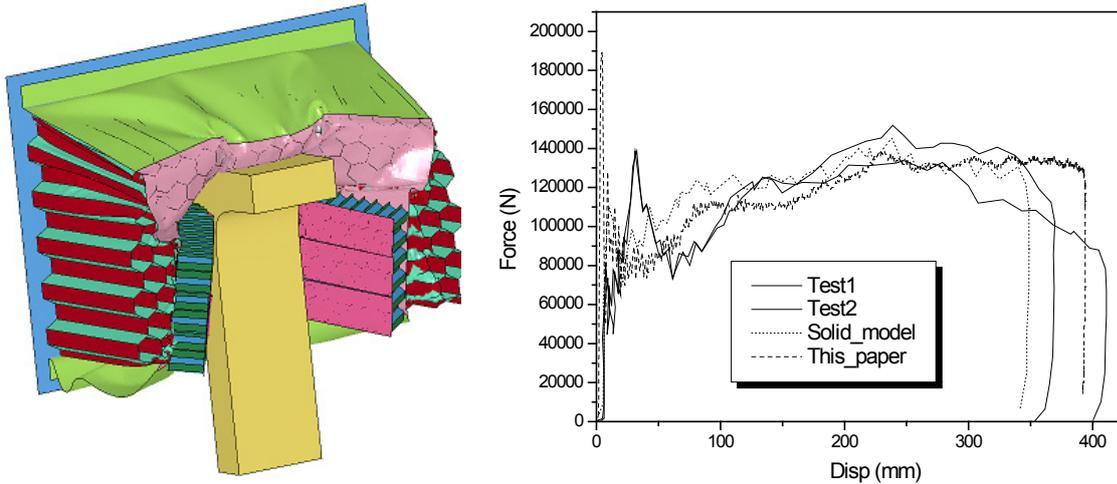
Fig. 11: Result of ODB impacted with vertical bar
