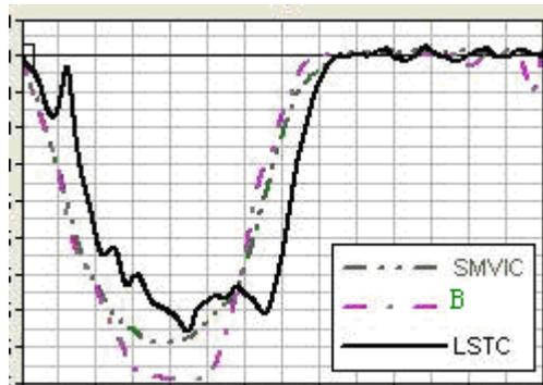
Fig. 14: Acceleration of trolley in side impact with a car
