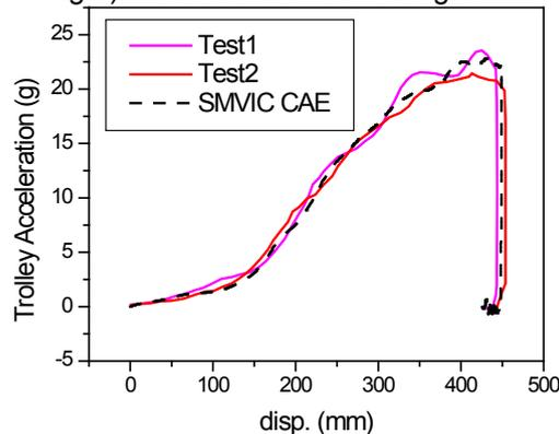
Fig. 7: Acceleration of MDB (Rigid sill loading test)
