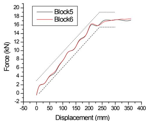
Fig. 3: Static strength of MDB (Block 5 & 6)
