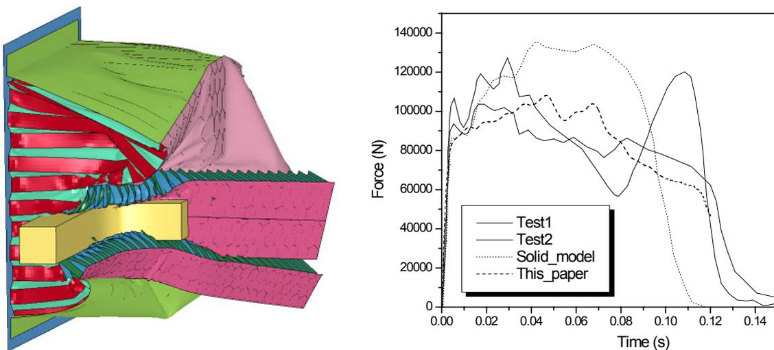
Fig. 10: Result of ODB impacted with lower bar
