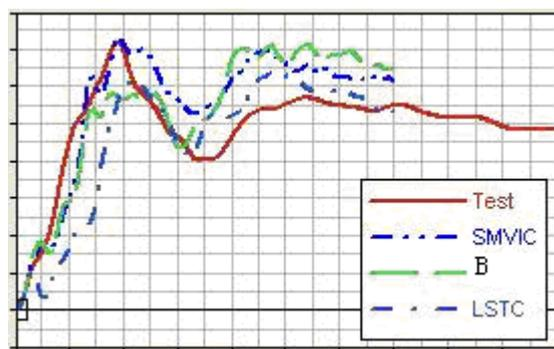
Fig. 15: Intrusion of B-pillar in side impact
