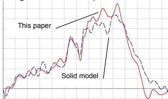
Fig. 13: B-pillar Acceleration of a car in ODB frontal crash
