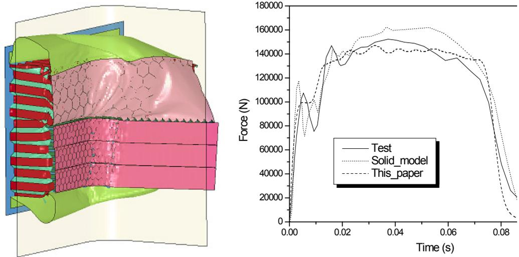
Fig. 9: Result of ODB impacted with half wall
