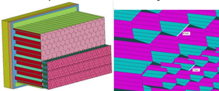
Fig. 1: Shell element model of ODB honeycomb of this paper
