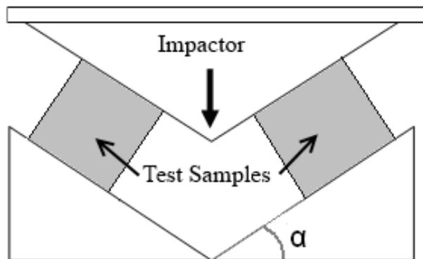
Figure 3. Off-Axis crush test arrangement
