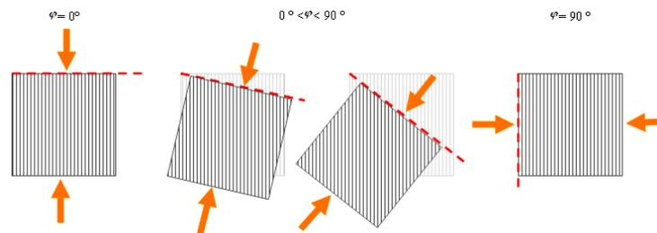
Figure 2. Static angled compressive test procedure
