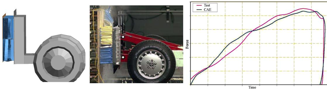
Figure 6. Load-Cell test and FE model
