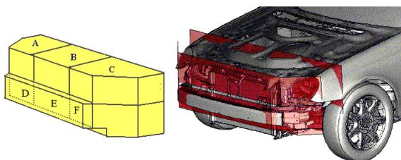
Figure 1. AE-MDB compared to the front part of a car
