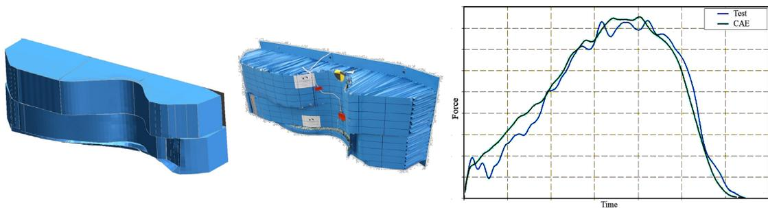
Figure 7. Offset-Pole test and FE model
