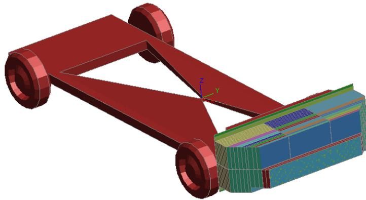
Figure 4. AE-MDB FE model
