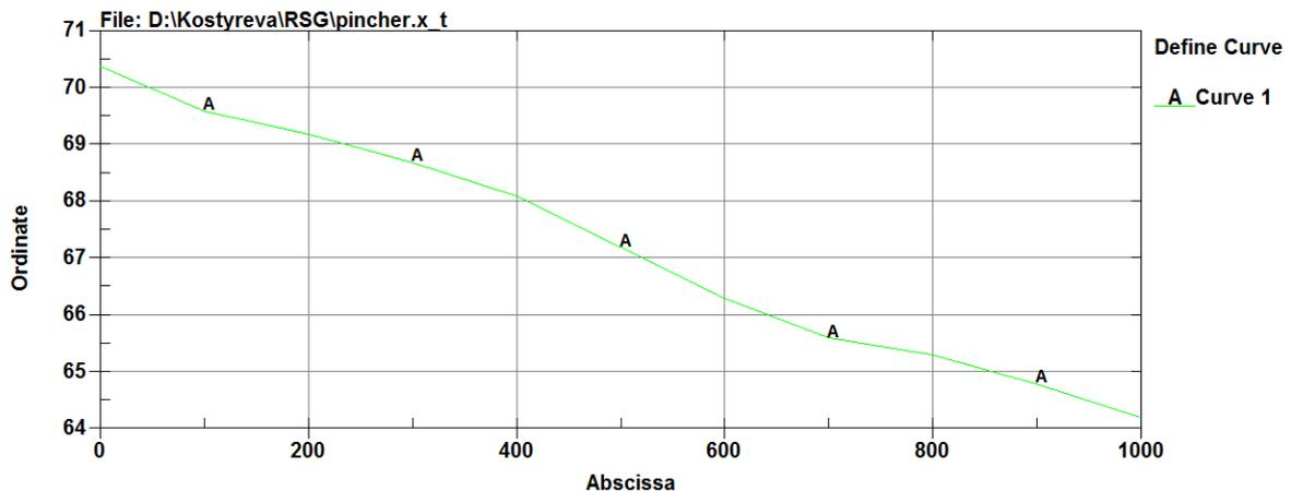
Fig. 7. Heat transfer coefficient during pincher movement.
