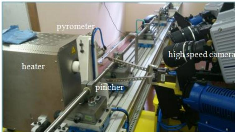
Fig. 2: Scheme with separate heater
