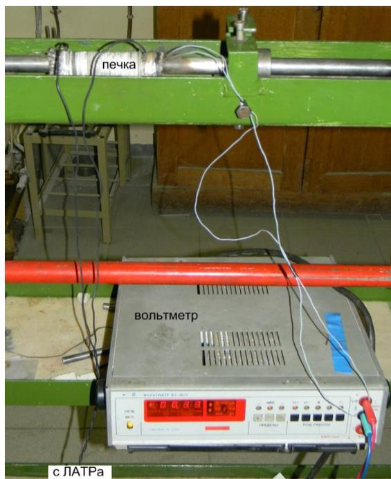
Fig. 1: Heater placed on the rods
