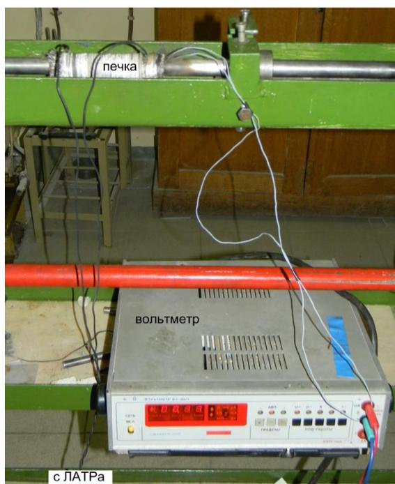
Fig. 1: Heater placed on the rods
