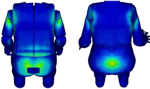
Fig. 13 Contact pressure between occupant and carbon fibre seat
