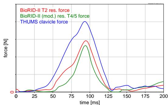
Fig. 25 Left shoulder forces (carbon fibre seat)
