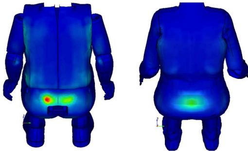
Fig. 18 Contact pressure between occupant and vehicle seat
