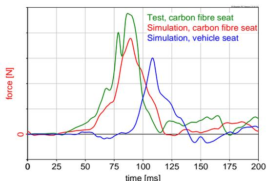
Fig. 27 Differential upper neck shear force (BioRID-II)
