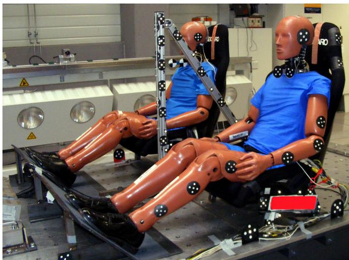
Fig. 1 Set-up of the BioRID-II evaluation tests
