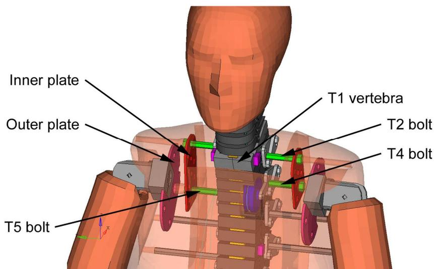
Fig. 6 Shoulder design of the BioRID-II (model release 3.0)
