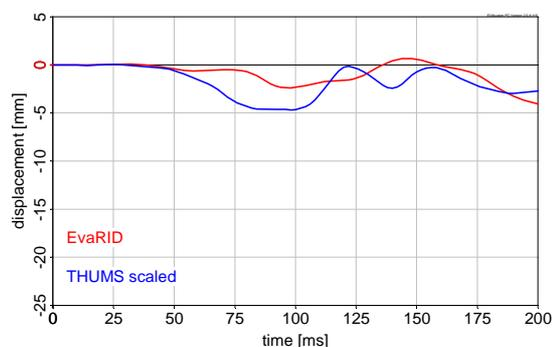
Fig. 24 Lateral compression of the shoulders (standard vehicle seat)
