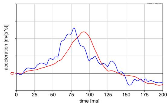
Fig. 12 Pelvis acceleration (x)
