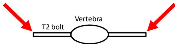
Fig. 29 Schematic diagram of the distribution of BioRID-II shoulder loads
