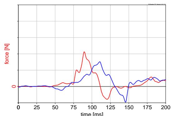
Fig. 28 Differential upper neck shear force (EvaRID)
