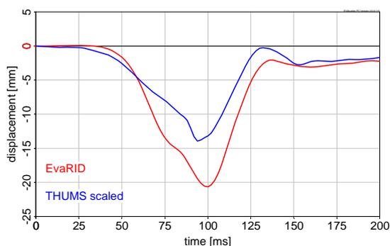
Fig. 23 Lateral compression of the shoulders (carbon fibre seat)
