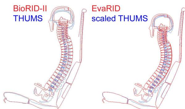
Fig. 3 Posture of BioRID-II, THUMS, EvaRID, and downscaled THUMS (carbon fibre seat)
