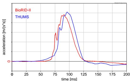
Fig. 9 Head acceleration (x)
