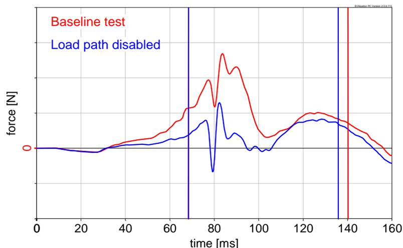
Fig. 2 Upper neck shear forces – baseline test and test with disabled load path
