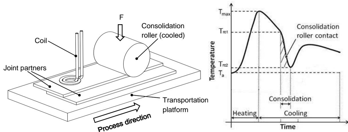
Fig. 2: a) Experimental test-bed setup for the continuous induction welding of two material partners and b) corresponding example thermal profile on the top surface of the joint
