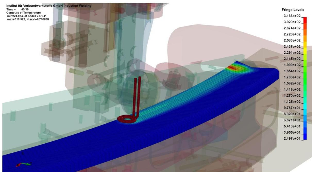
Fig. 12: Large demonstration model of the KUKA robot at the Institut für Verbundwerkstoffe GmbH performing an induction welding procedure on an automotive component
