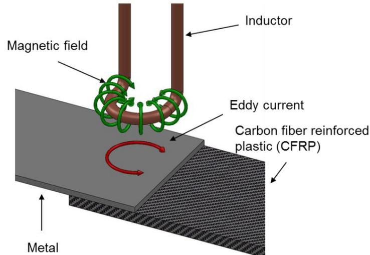
Fig. 1: Working principle of induction heating (image courtesy of Mrs. Mirja Didi IVW GmbH)
