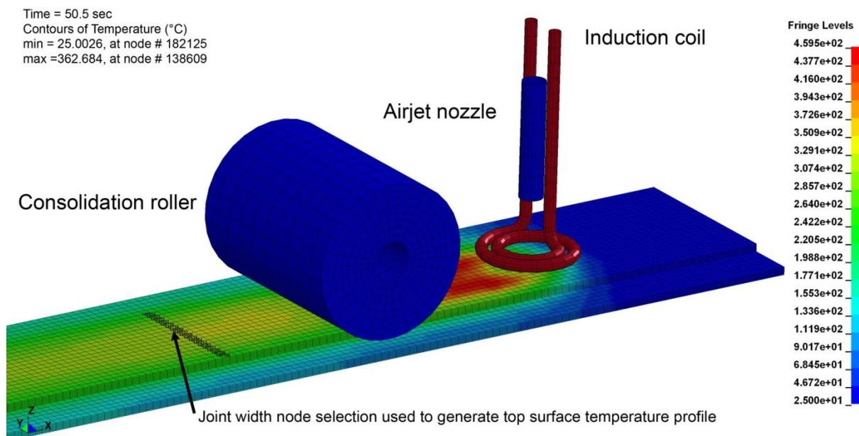
Fig. 4: Induction welding simulation test-bed developed using LS-DYNA® (R7) and the wealth of knowledge accumulated at the Institut für Verbundwerkstoffe GmbH over the last 15 years
