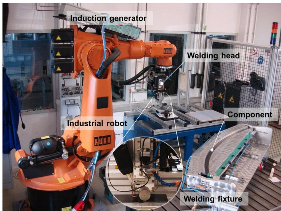
Fig. 3: Industrial continuous induction welding setup using a KUKA robot at the Institute für Verbunwerkstoffe GmbH
