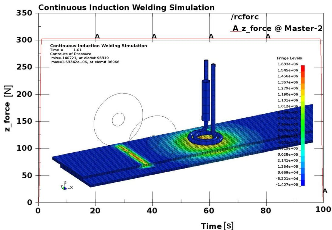
Fig. 5: Induction welding simulation test-bed showing the overall roller contact force together with contours of pressure in the laminate generated as a result of roller contact and air-jet pressure
