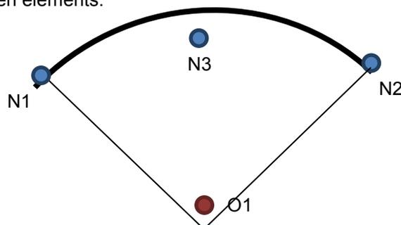
Fig. 2: Pipe beam node orientation.
