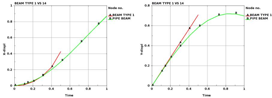
Fig. 4: To the left is the x-displacements for the elbow (B) beam and beam type 1 (A) shown. To the right is the y-displacements for the elbow beam (B) and beam type 1 (A) shown.
