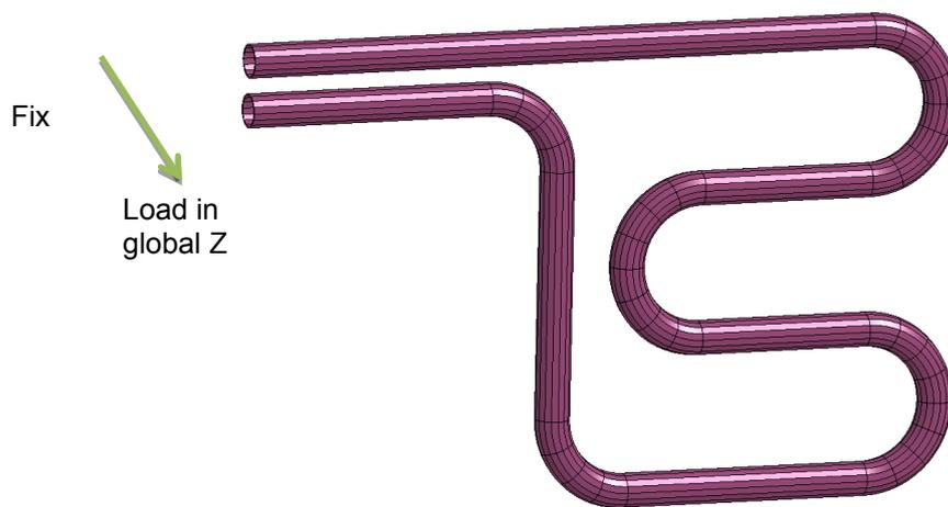
Fig. 6: Initial model. Node 1 is fix and the last node is loaded in the global z-direction.
