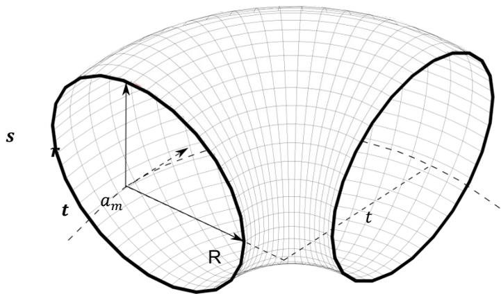
Fig. 1: Illustration of a pipe beam element,  $r$ ,  $s$  and  $t$  are position vectors,  $a_m$  is the mean radius of the tube,  $R$  is the pipe curvature radius and  $t$  is the wall thickness.
