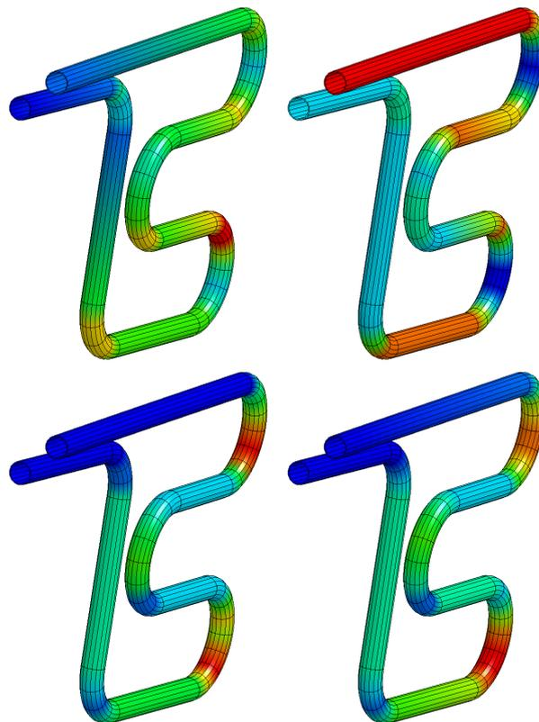
Fig. 7: Different fringe plots. Reading from top left to bottom right: axial-stress, loop-stress, rs-stress and tr-stress.
