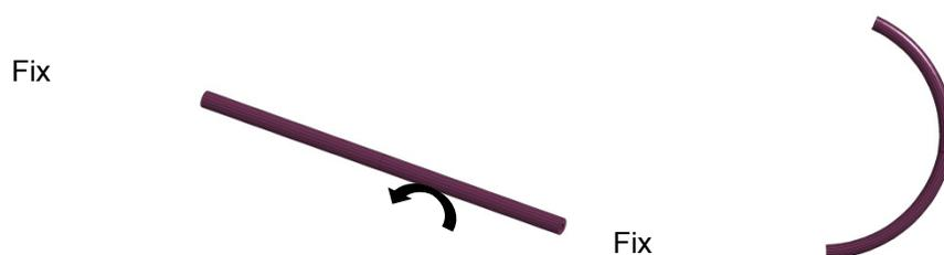
Fig. 3: Cantilever beam modeled with 2 elbow elements. To the left is the initial geometry and to the right is the deformed state.
