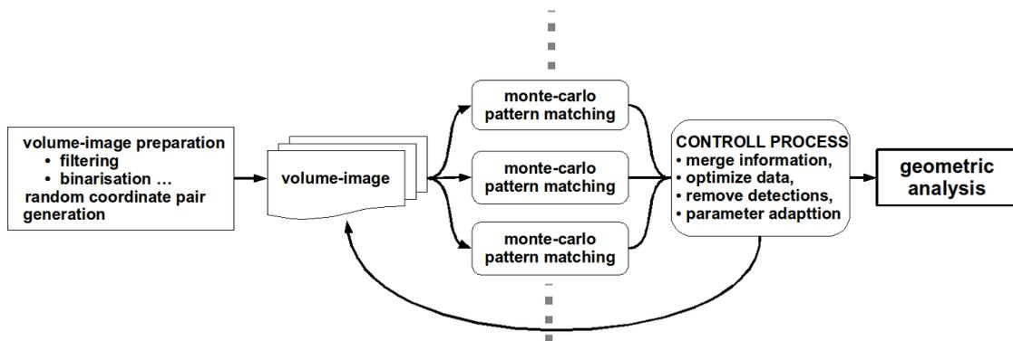
Figure 14: Flow chart of the new fibre analysis algorithm
