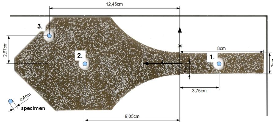
Figure 18: Specimen positions 1,2 and 3 in the part
