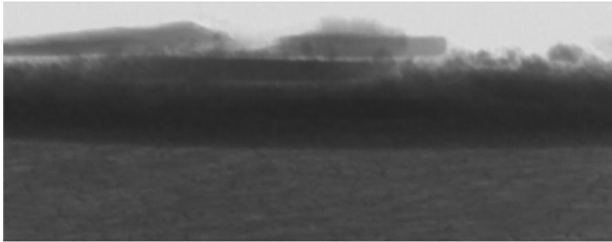
Figure 11:  $\mu$ CT picture, dense paint and paint flakes clearly visible
