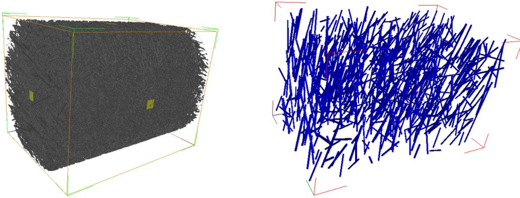
Figure 15: 3D scan results of PA6GF30 (some matrix removed for visibility)      Figure 16: Detected fibres in PA6GF30 (only 10% shown)
