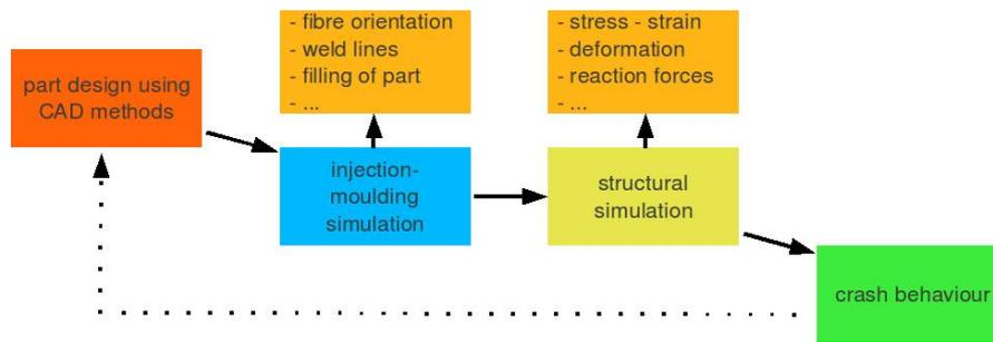
Figure 3: Processchain “integrative simulation”
