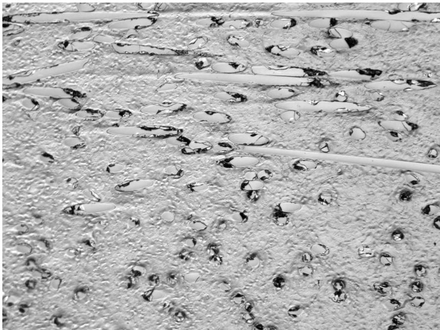
Figure 5: Glas fibre ellipses in a test specimen
