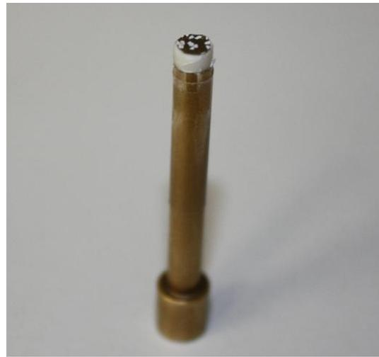
Figure 10:  $\text{Ø } 4\text{ mm}$  specimen on mount
