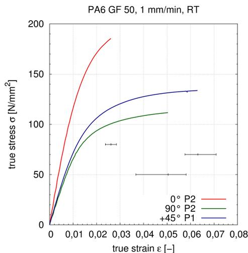
Figure 2: PA 6 GF 50% under different loads
