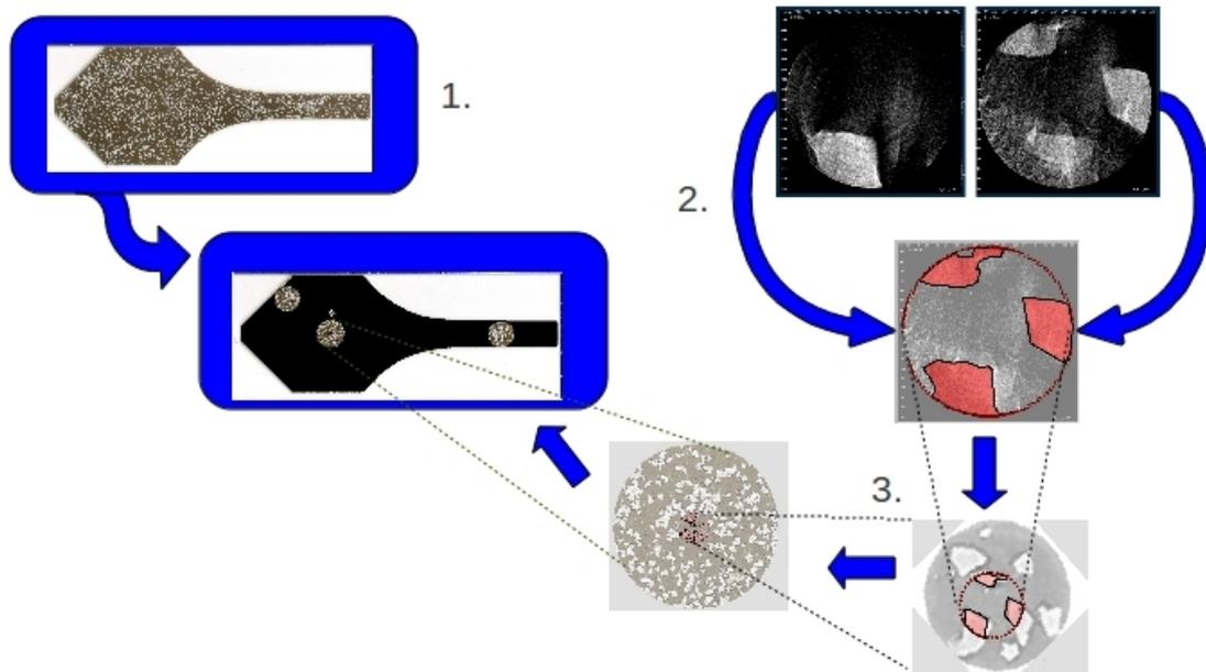
Figure 12: Positioning and reorientation using special paint
