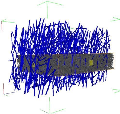
Figure 17: 3D scan results of PA6GF30 overlaid with detected fibres
