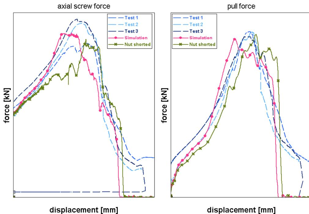
**Fig. 14: Comparison test with simulation with shorted nut – force vs. displacement**
