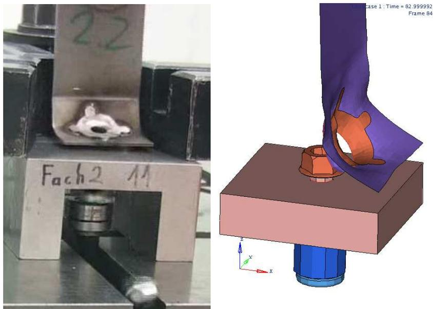
Fig. 7: Left picture: failure of screw in test. Right picture: peeling in FEA
