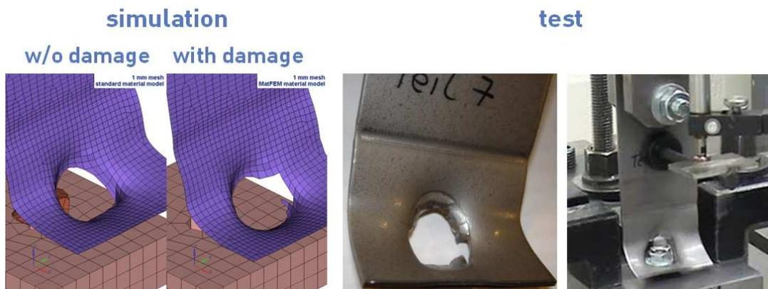
Fig. 11: Comparison of simulation with test after failure.
