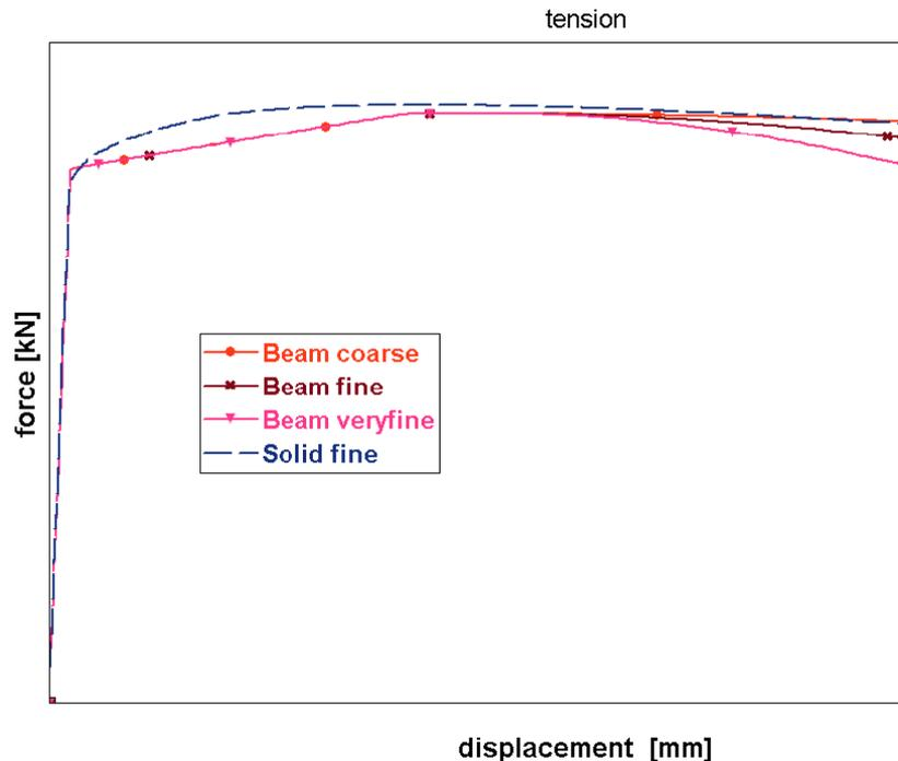
**Fig. 3: Force vs. displacement under tension load**
