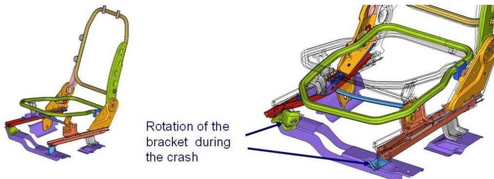
**Fig. 1: Deformation of screw connections on seat structures**
