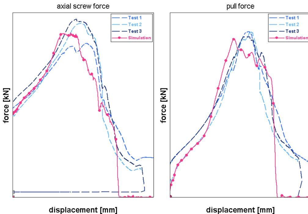
**Fig. 12: Comparison simulation with test results – force vs. displacement**
