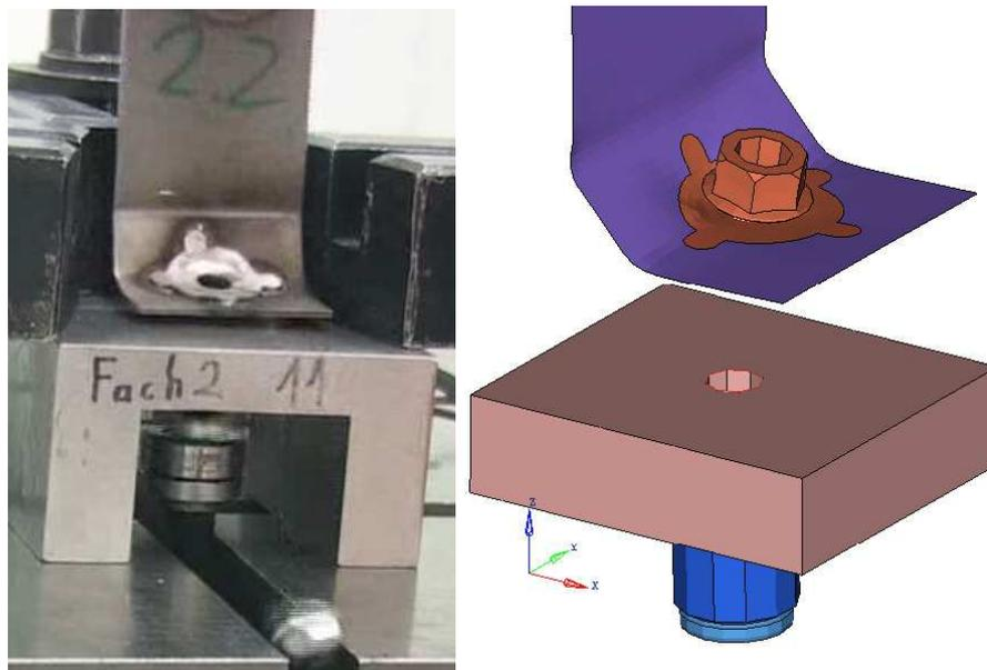
Fig. 16: Failure of screw in test and simulation
