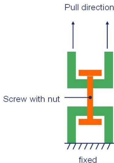
Fig. 8: Test configuration for material detection test.
