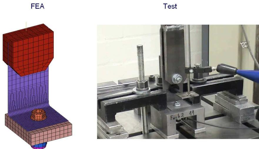
Fig. 10: Test configuration for screw validation test
