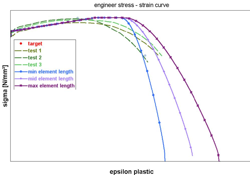
**Fig. 9: Validation of material card -  $\sigma$  vs.  $\epsilon_{plast}$**
