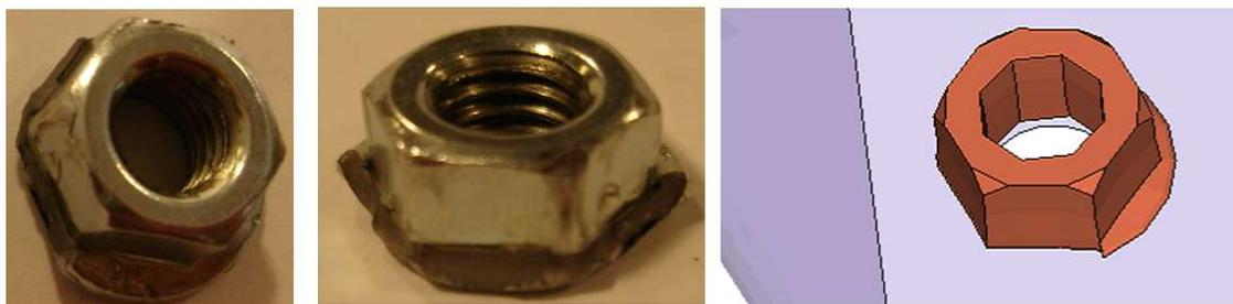
**Fig. 13: Deformation of nut after test and reduced nut in FEA**
