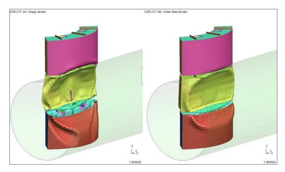
It can be seen that the deformation is significantly reduced when the effects of the water are included. Animations of the water filled analysis show the water being forced out of the holes during the impact. An analysis with only two quadrants, where the water is ejected upwards, shows this even more clearly.
