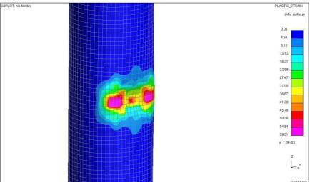
This amount of deformation and the high strains associated would be sufficient to cause collapse of the structure and as such a fender system is required to absorb the energy.
