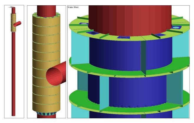
The image on the left shows the full model with rigid ties to two points at the top and centrally at the base.
