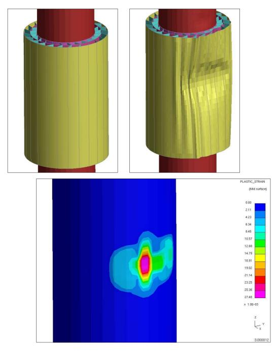
This shows that the strain in the platform leg has been reduced from 6% over a large area to 2.7% over a much smaller area. To further reduce the strains in the platform leg and to reduce the reaction forces at the top and bottom of the platform leg the effects of water within the fender were included.
