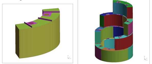
The fender system is formed from these hollow quadrants which are 1m thick and 2m high. They are constructed from 12mm thick steel with two holes in the top surface which are designed such that the amount of water that can flow through them is such that it will decelerate the ship at a constant rate. These quadrants are welded around the platform leg and separated vertically by supports on the top face to allow the water to flow out between them.
