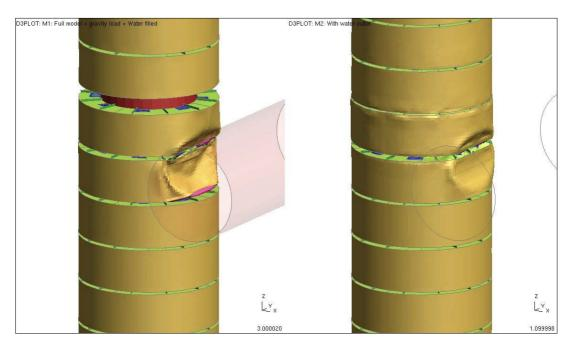
As would be expected, the deformation of the water filled fender, shown on the right, is substantially less than those of the dry fender, shown on the left.
