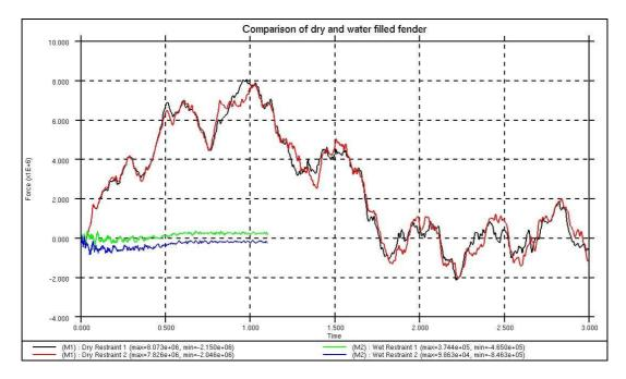
The impact duration for the dry fender (1.1 seconds) is much longer than for the water filled fender (0.5 seconds). The reaction forces at the restraints are significantly reduced by the inclusion of the water in the fender. The dry fender peak reaction force is 8.1MN compared to the water filled fender peak reaction force of -0.8MN.
