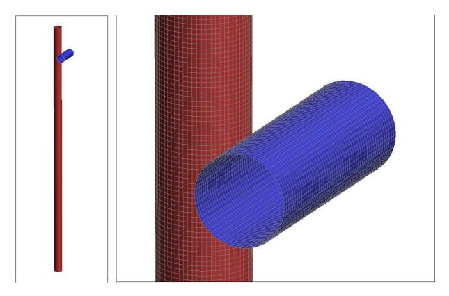
The platform leg is approximately 136m long, 4.5m diameter and 76mm thick. High order thin shell element have been used for all analyses. The ship strikes the platform leg and all energy is transferred from the ship to the platform leg. The final deformed shape and associated plastic strain is shown in the figure below.
