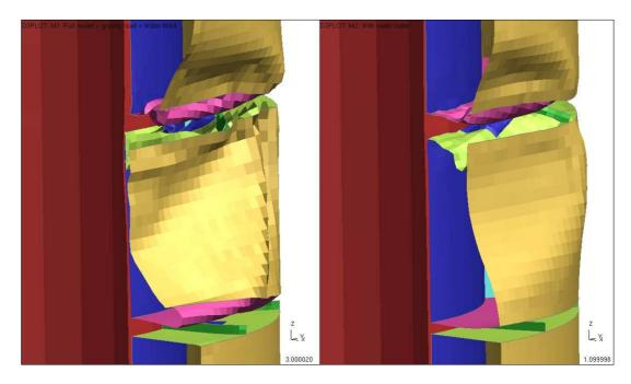
A cross section at the point of impact shows that the dry fender has completely compressed and damage is observed in the main platform leg, however, in the water filled fender system the platform leg remains undeformed.
