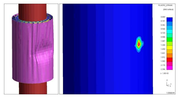
The plastic strain in the platform leg is now a localised surface strain of 0.2% which will not cause collapse in the leg. In addition the reaction forces observed at the top and base of the platform leg are reduced by the introduction of the water in the analysis as energy is dissipated in moving the water.
