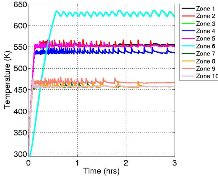
Figure 4: Temperature evolution in the 10 separate die zones for the first step
