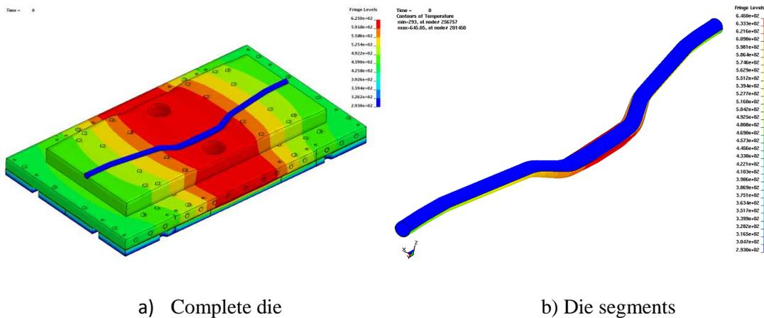
Figure 5: Temperature distribution in the heating die at the beginning of the second step
