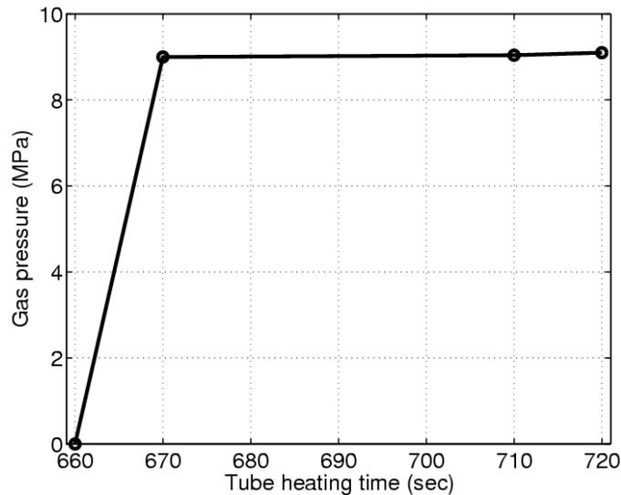
Figure 8: Applied gas pressure curve
