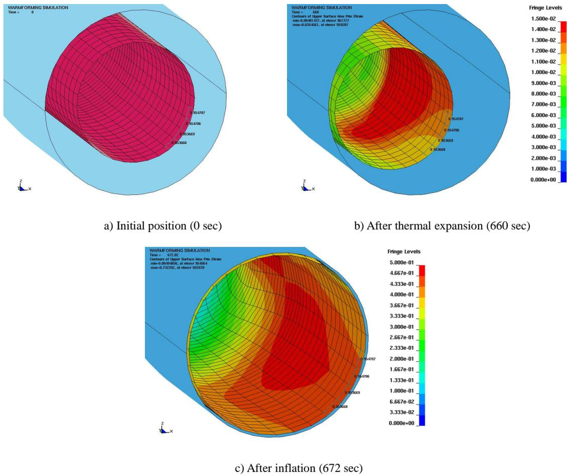
Figure 10: Strains at the lengthwise middle of the tube during warm forming
