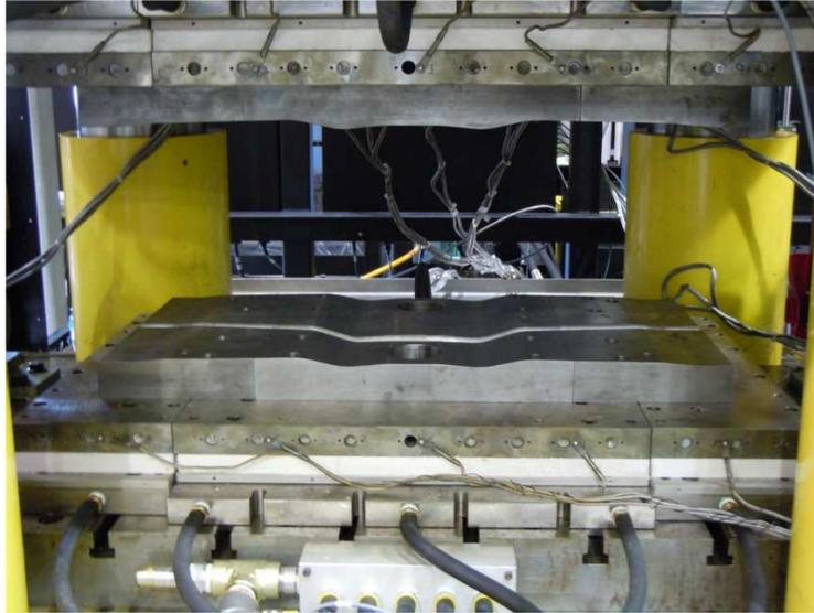
Figure 1: Heating die for warm tube forming
