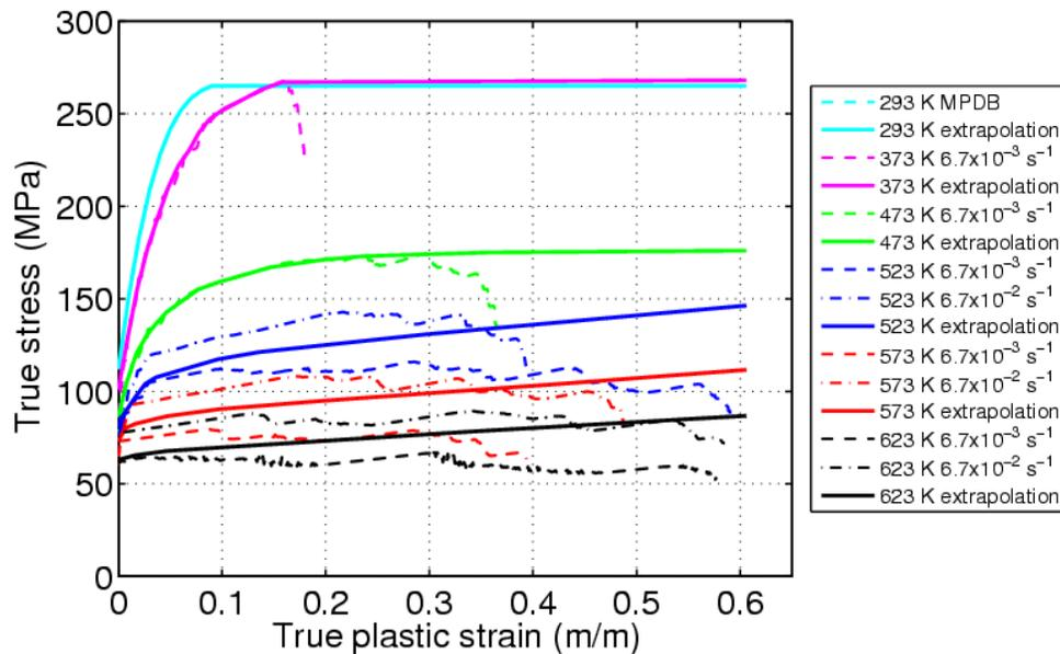
Figure 7: Measured and extrapolated curves for 7075 aluminium alloy at different temperatures
