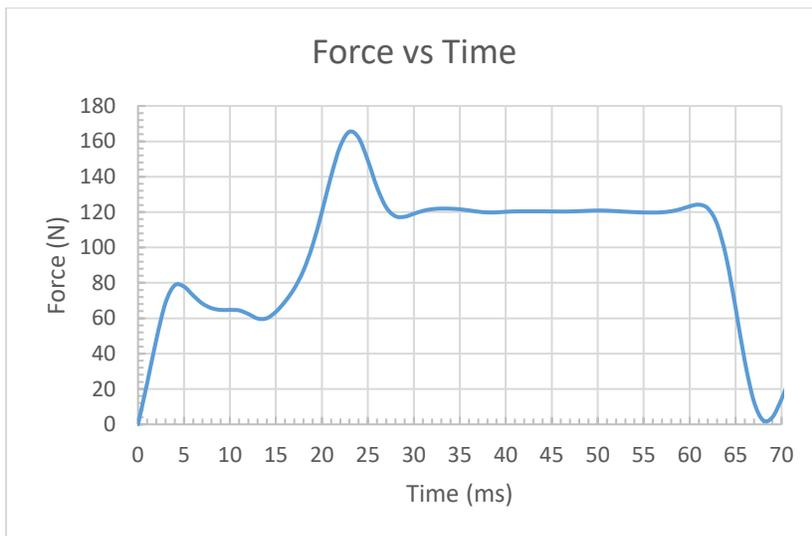
Figure(3) is the Force (N) vs time (ms) graph. The indenter observes a maximum resistive force of 165N
