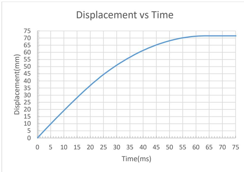
Figure(2) is the displacement (mm) vs time (ms) graph. The indenter comes to rest at 65ms after travelling a depth of 72 mm.
