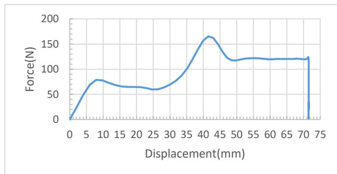
Figure(1) is the Force (N) vs Displacement (ms) graph. Zone I is the Densification zone and Zone II is the Plateau region
