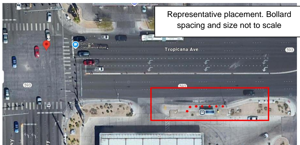
Figure 1. A possible layout of bollards at a bus stop at a major intersection [3].
