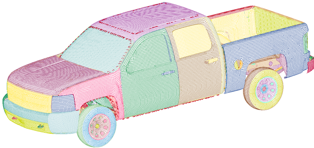
Figure 4. FEA model of 2007 Silverado, course mesh (CCSA, 2016).
