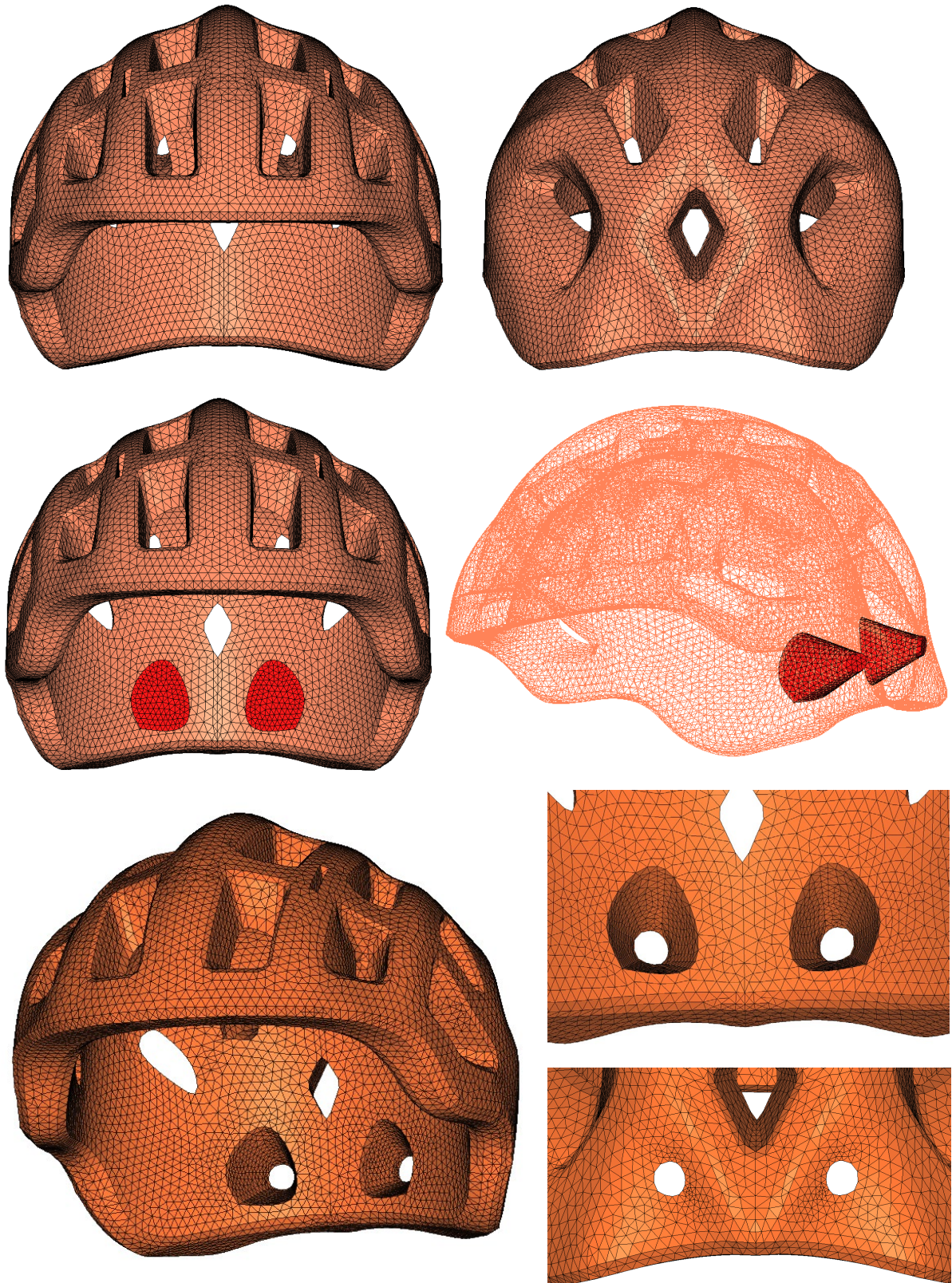
Figure 7: View of the helmet initial (top) and final (bottom) mesh when using DEP MeshWorks boolean operation feature to add a specific shape hole (middle) directly in a volumetric mesh
