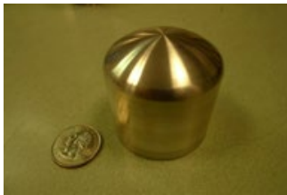
Fig.8: Projectile used in impact tests.
