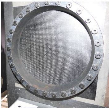
Fig.9: Composite plate used in impact tests.
