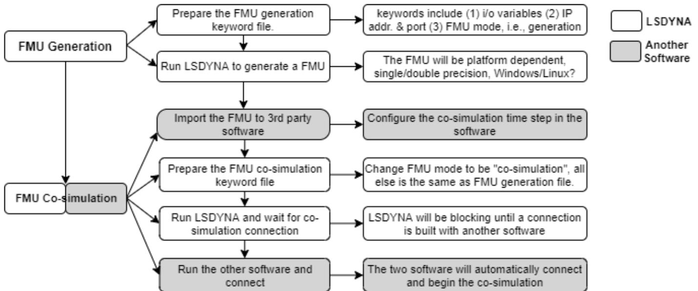
Figure 1. Flow Chart of LS-DYNA Co-simulation
