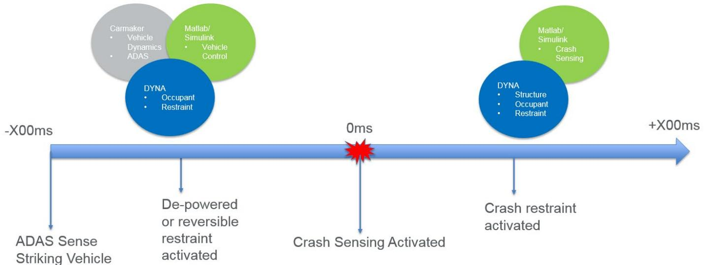
**Figure 8. Co-simulation Timeline of Integrated Sensing System**
