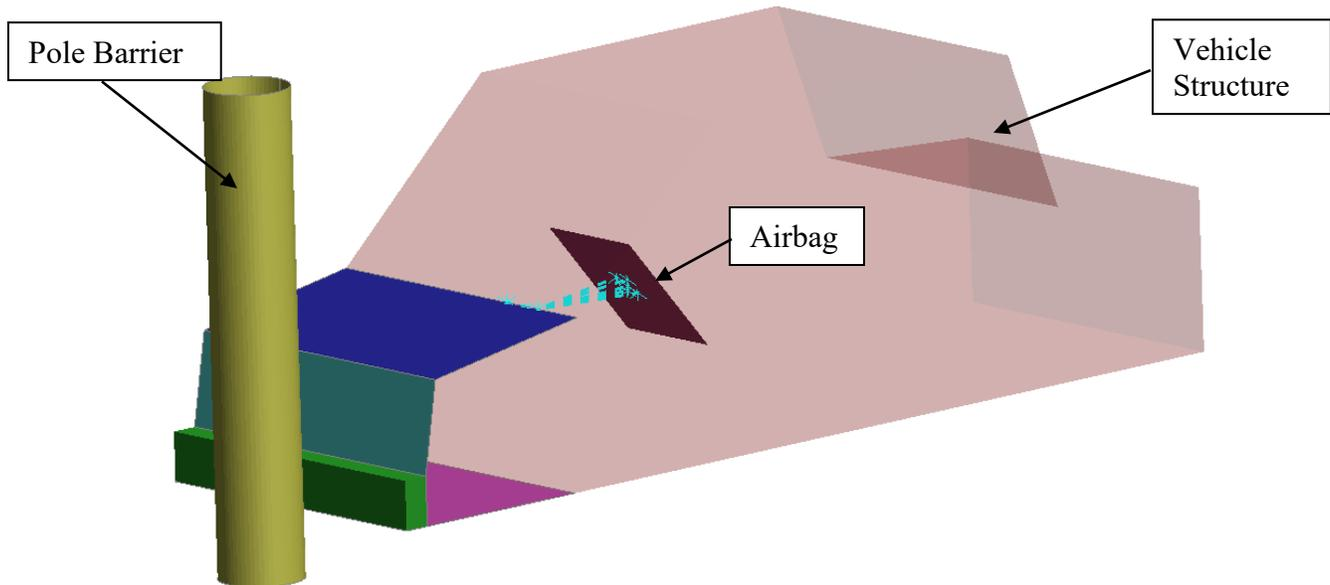
Figure 4. Simple Vehicle FE Crash Model
