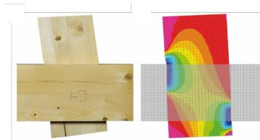
(b) Close-up deformation and stress contour – Simulation and experiment
