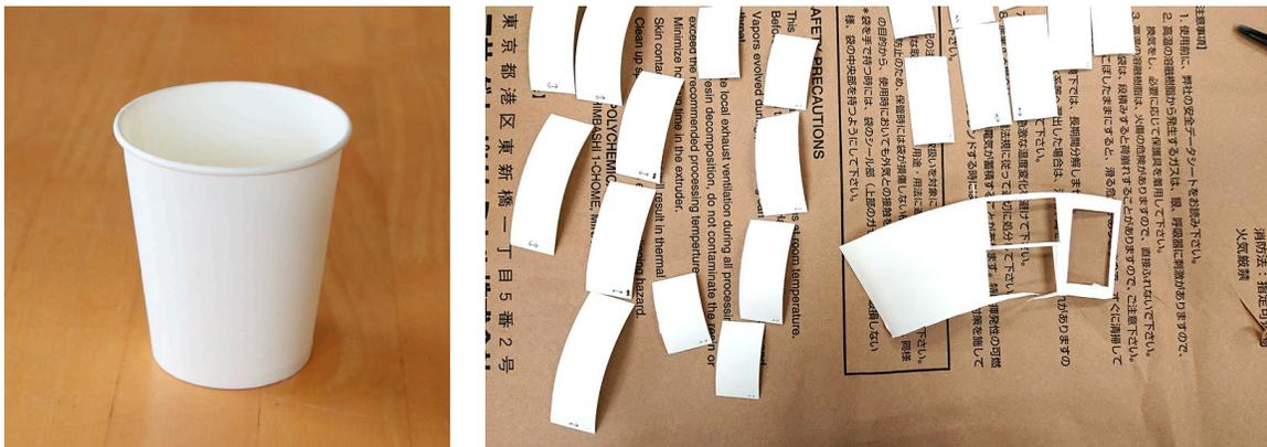
Fig.2 Paper cup and specimens
