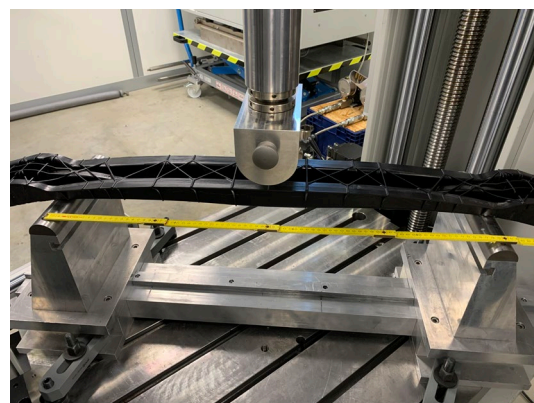
Figure 1b: Actual test setup for quasi-static testing of the front bumper beam.
