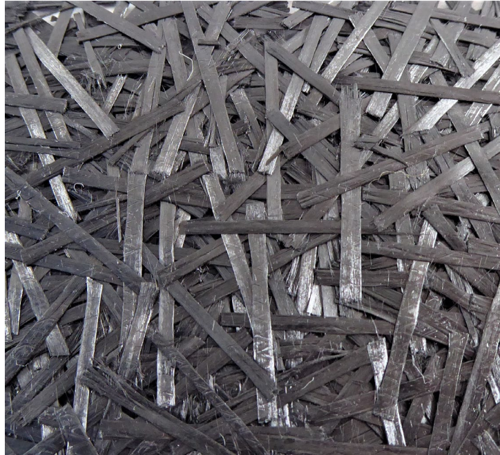
Figure 1: Prepreg platelet molding compound in sheet form
