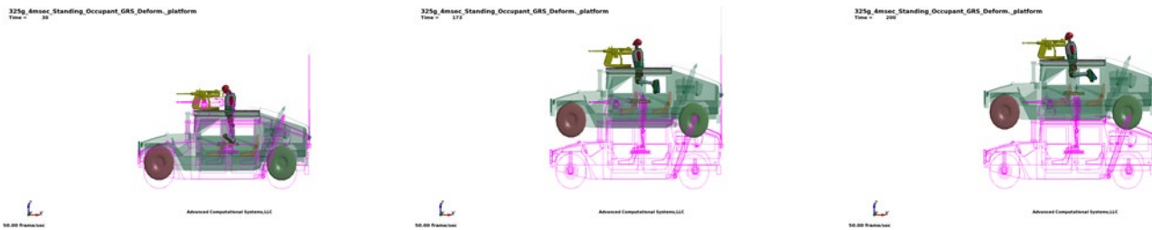
Fig. 23. Kinematics of the standing restrained occupant on 75mm height deformable platform.
