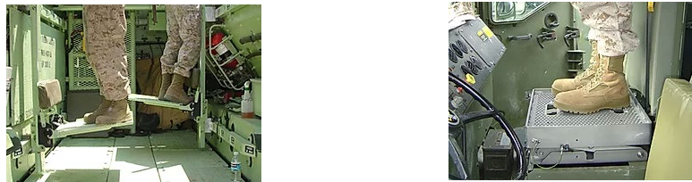
Figure 5. Energy Attenuating System [Ref. 9].
