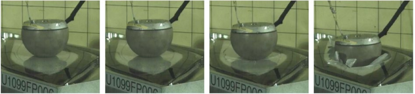
Figure 4 - Head impact test on side window for validation
