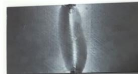
Buckling mode of compression after impact (CAI) test.
