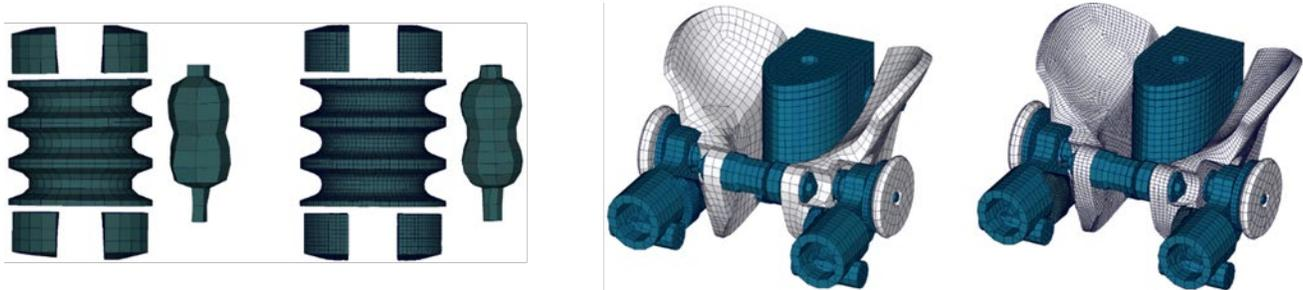
Figure 5: Comparison of old (left) and new mesh (right) of neck/neck buffers and iliac wings
