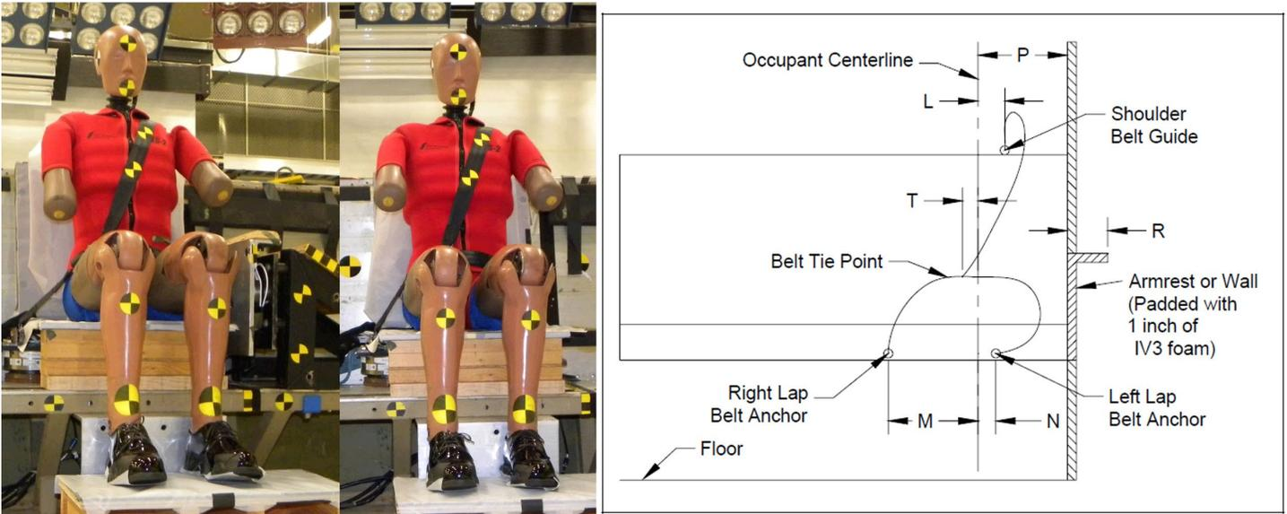
Figure 1: ARP 5765 sled test setup with armrest (left), without armrest (mid) and belt scheme (right) [1]
