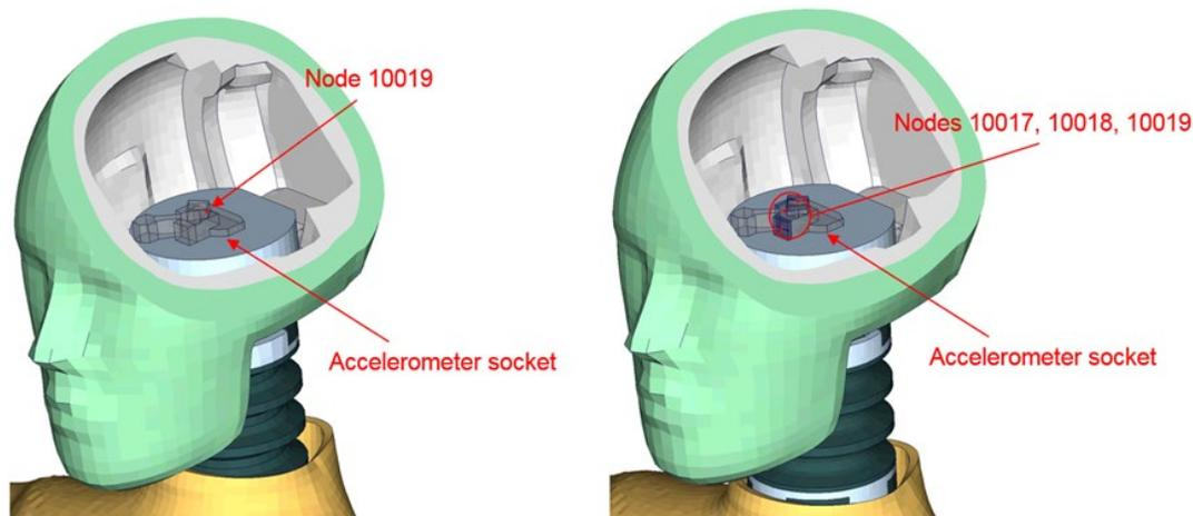
Figure 6: Comparison of old (left) and new (right) head accelerometer positions
