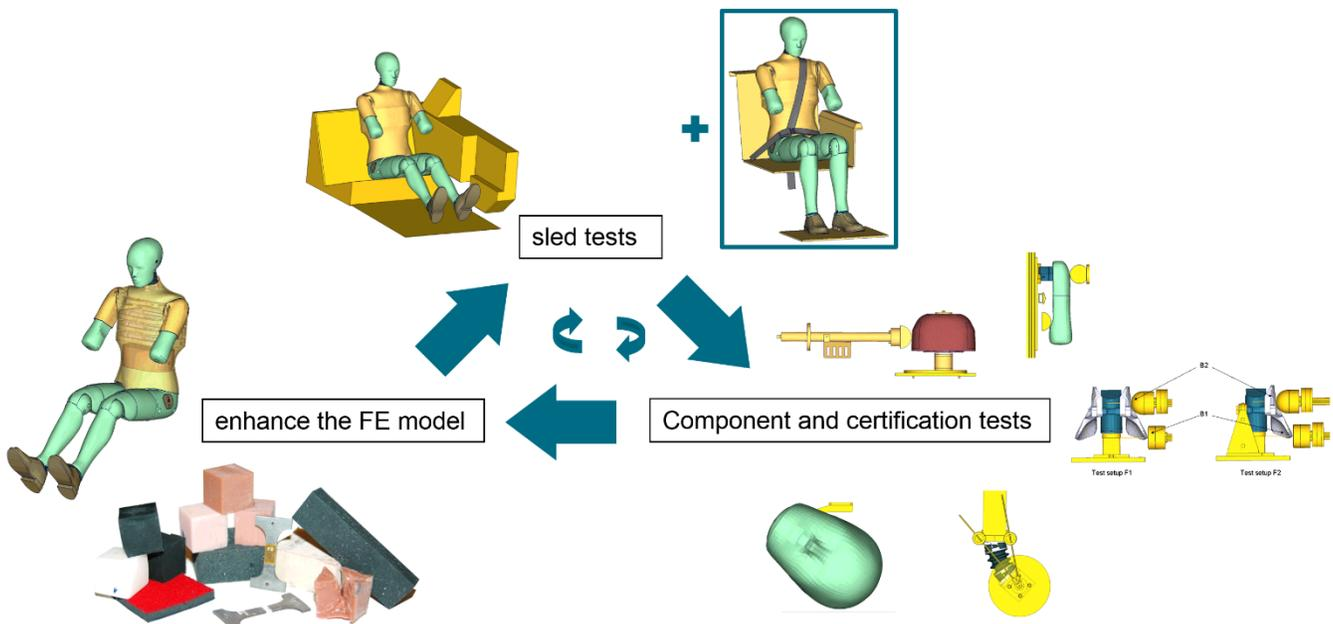
Figure 4: Methodology of dummy model updating
