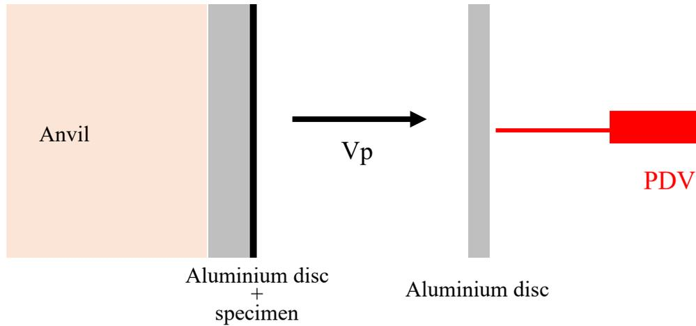
Figure 1 Reverse plate impact configuration
