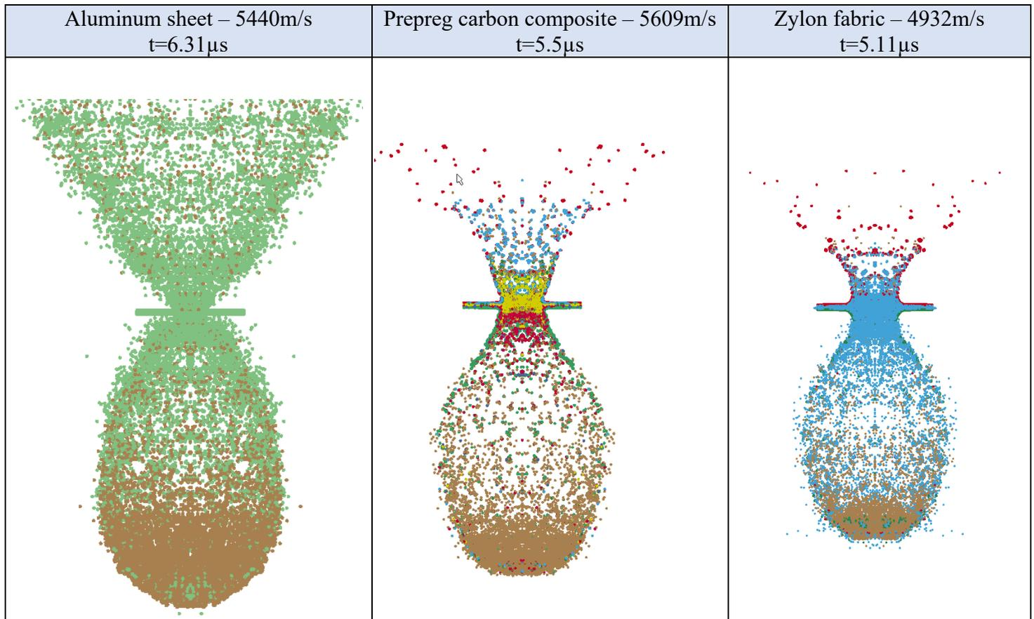
Figure 10 Qualitative behaviour comparison between numerical aluminum, prepreg carbon and zylon fabric under HVI at ~6km/s
