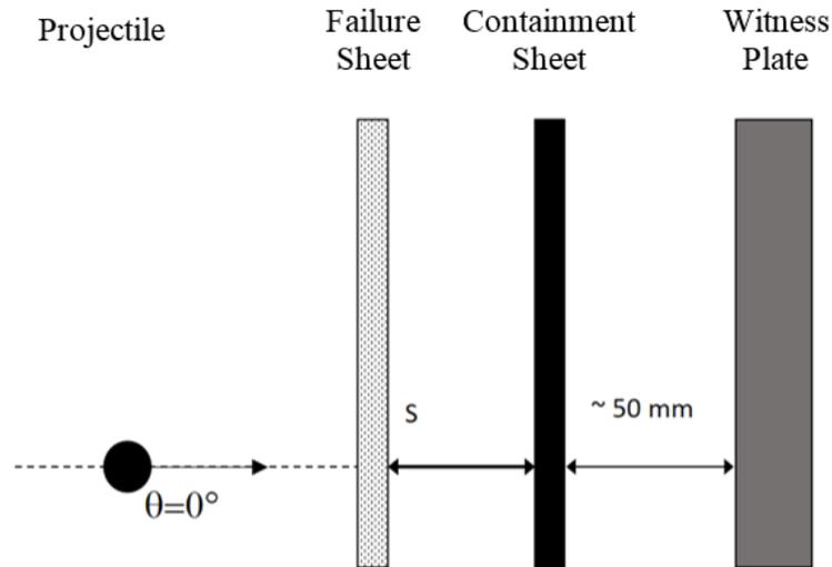
Figure 4. Initial configuration of the target
