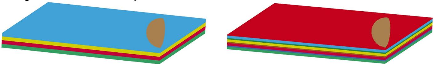
Figure 6 Models of prepreg carbon composite: four homogeneous plies in the plate (left) and modelling of resin intermediate layers (right)
