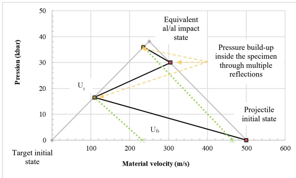
Figure 2 Representation of multiple shock wave reflections inside the specimen
