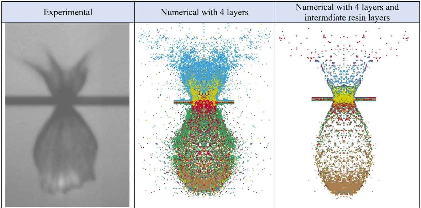
Figure 8 Picture of the impact result on the experimental plate (left), on the 4 homogeneous plies model (middle) and on the resin intermediate layer modelling model (right) taken at the same time
