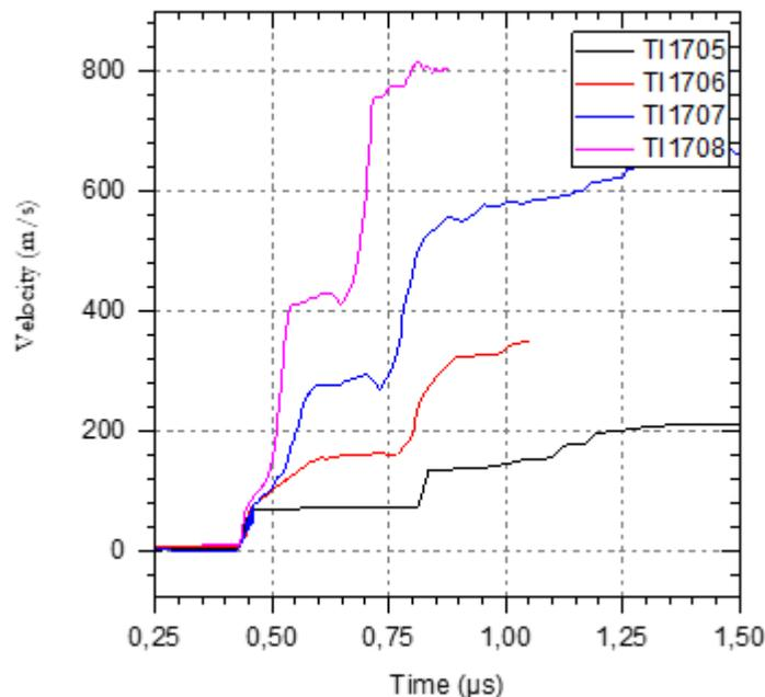
Figure 3 Aluminum target free surface velocity profile
