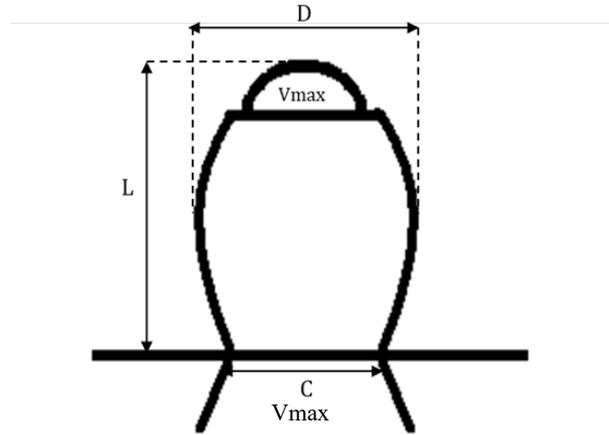
Figure 7: Illustration of the profile measurements
