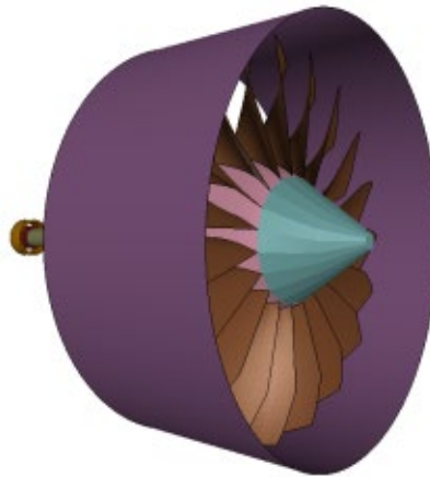
Figure 5 Rotating engine prior to blade out
