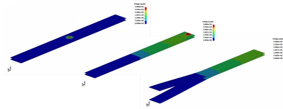
Fig.4: Welding and subsequent loading of two sheet metals. From left to right: Temperature fields at beginning of the welding step, at the end of the welding step and after mechanical loading. Separation prohibited in heat affected contact zones.
