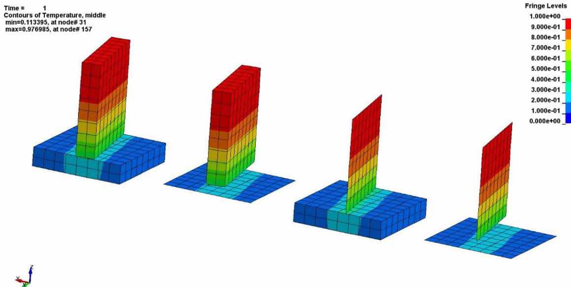
Fig.2: Validation test cases for shell edge thermal contact, resulting temperature distribution.
