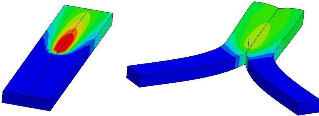
*Fig.3: Welding and subsequent loading of a butt weld of two bars. Temperature field at the end of the welding step is shown (left). Loading only results in a separation of the contact areas that have not been affected by the heat.*
