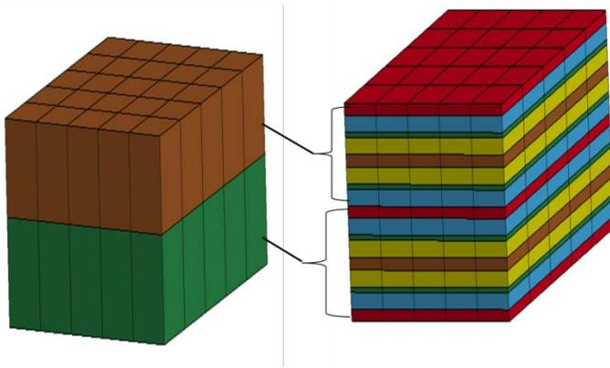
Fig.5: Tshell mesh provided by the user on the left and reconstructed EM/thermal mesh based on the composite lay-up in the Tshell elements on the right.
