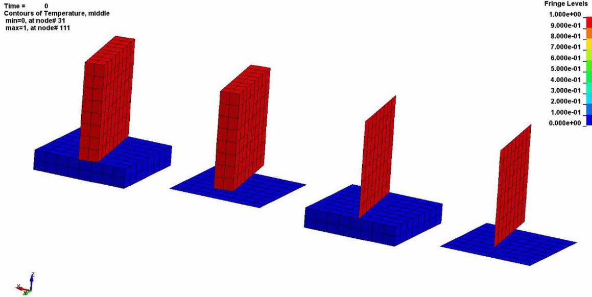
Fig.1: Validation test cases for shell edge thermal contact, initial temperature distribution.
