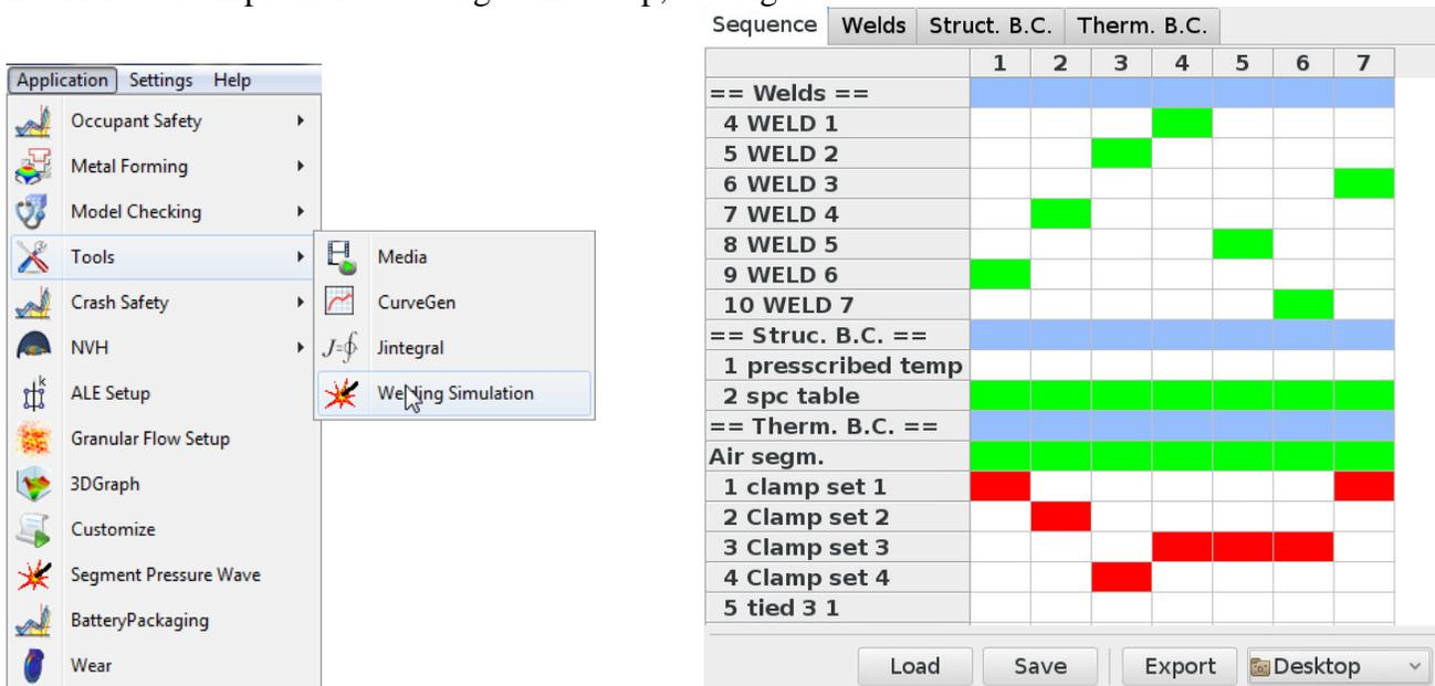
Figure 1: LS-PrePost welding GUI application and process window
