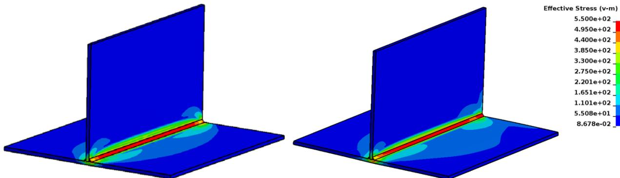
Figure 8: Von Mises stress from thermal dumping simulation (left) and incremental simulation (right)
