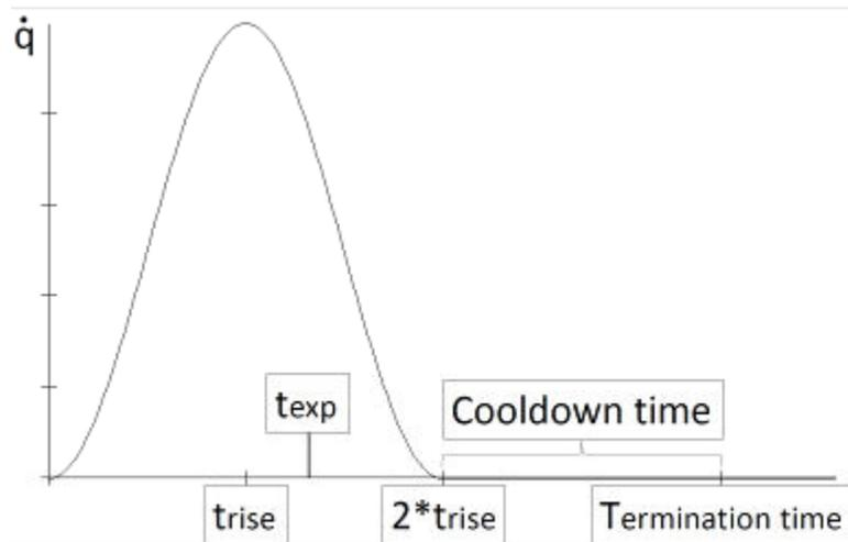
Figure 3: Thermal dumping weld energy approach and time definitions
