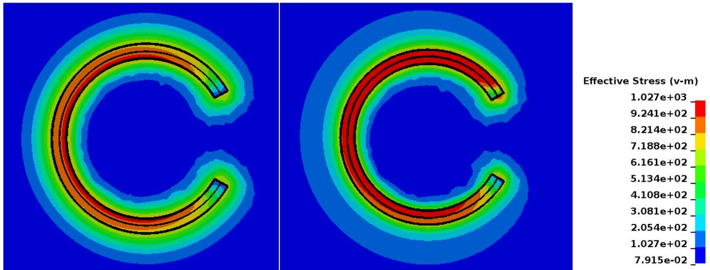
Figure 11: Resulting von Mises stress distribution after cooling of layer 3 for dumping methodology (left) and incremental (right)
