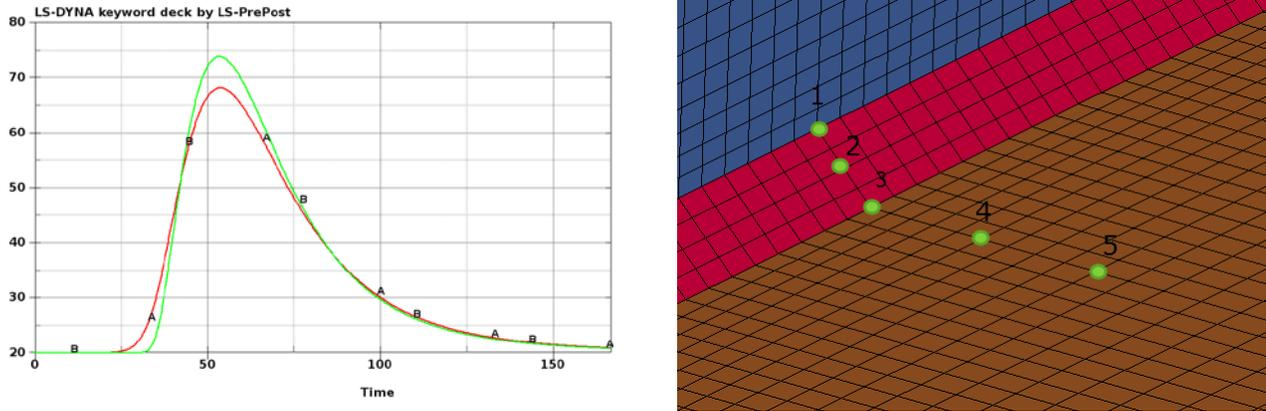
Figure 6: Temperature comparison in selected points. Red is incremental, and green is thermal dumping results.
