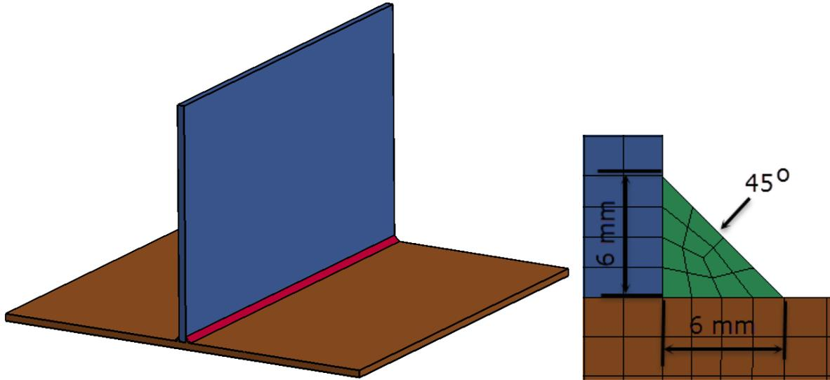
Figure 5: T-joint model
