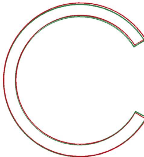
Figure 12: Resulting shape after cut off and spring back for dumping (green) and incremental (red)
