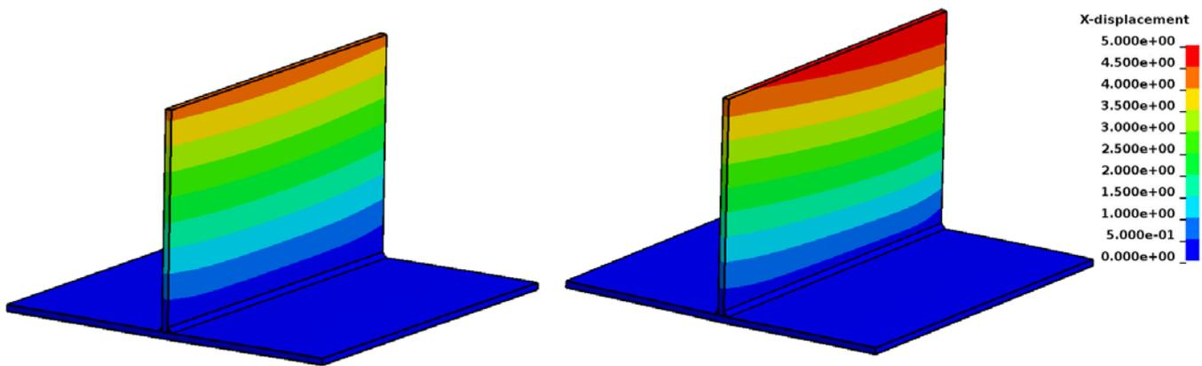
Figure 7: Tip displacement of thermal dumping simulation (left) and incremental simulation (right)
