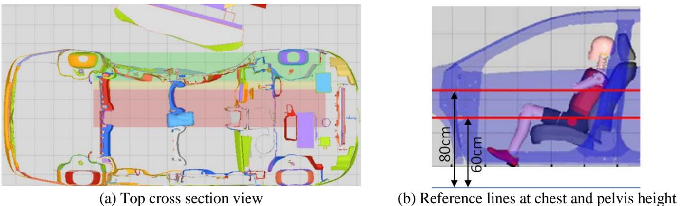
**Figure 6.** Example of structural intrusions measured horizontally at door outer
