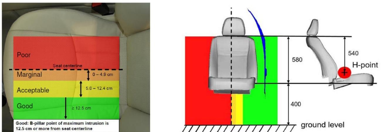
Figure 4. IIHS structural performance criteria, measured at the B-pillar
