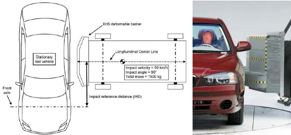
Figure 3. IIHS side impact configuration
