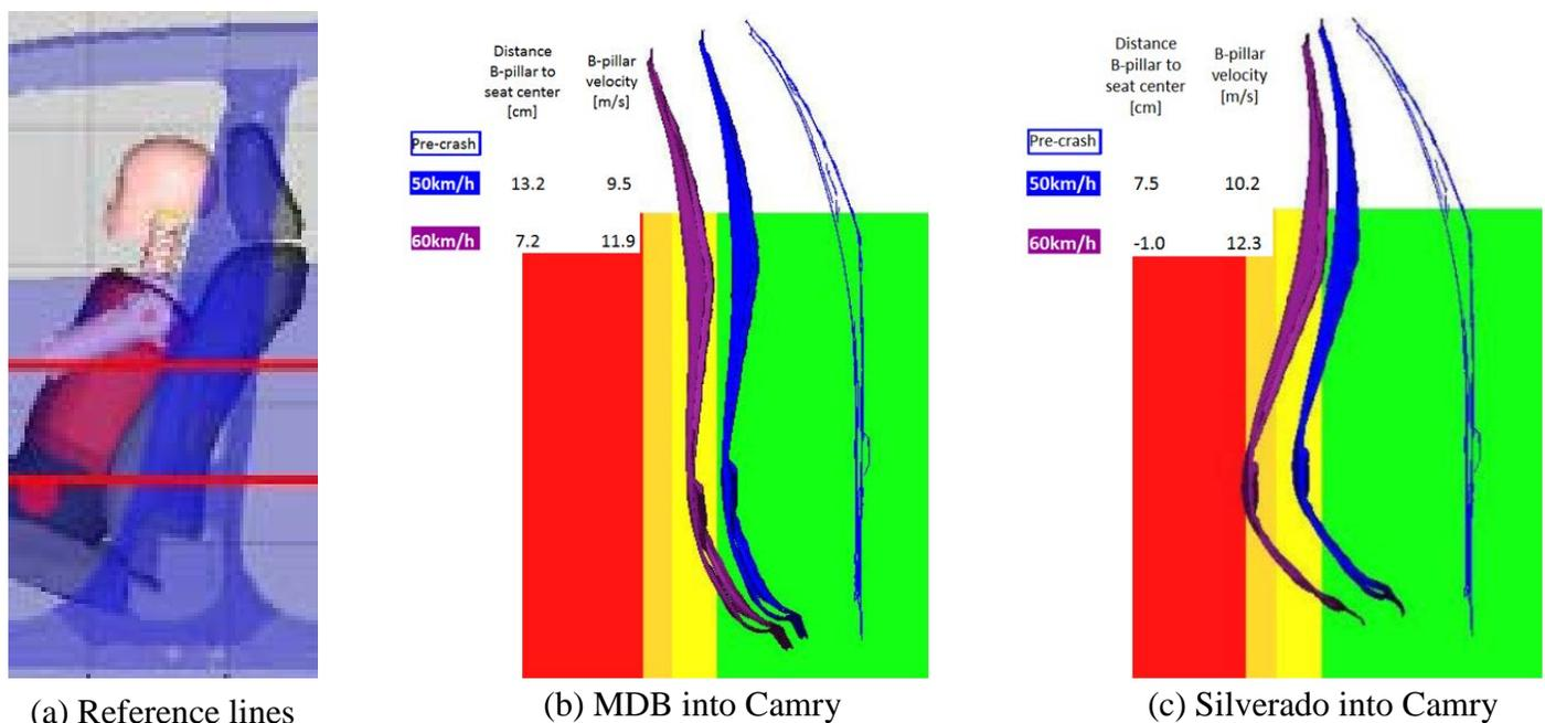
**Figure 7.** B-pillar deformation and velocity using different bullet vehicles and impact speeds
