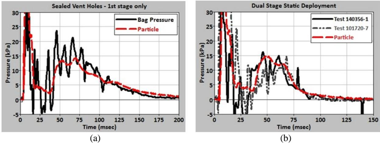
Figure 12. (a) The PAB first stage deployment with the vent sealed, (b) dual stage static deployment.
