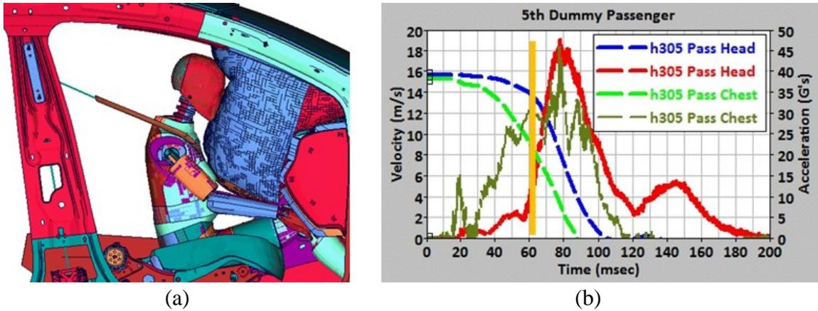
Figure 15. (a) GMX353 passenger simulation at 60msec, (b) The velocity and acceleration histories of the passenger's head and chest.
