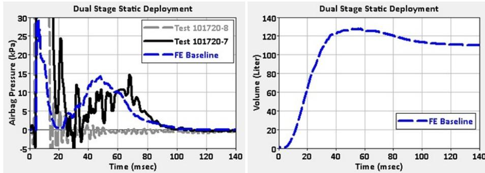
Figure 4. Dual stage static deployment correlation of the delivered PAB finite element model using GM internal HPC and LS-DYNA 971 version R6.1.2.
