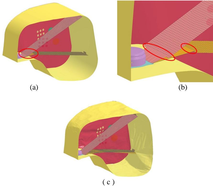
Figure 10. (a) The initial reference geometry of the PAB, (b) the second row of the nodes on the tethers near the inflator base were pulled toward the base at the end of the simulation, (c) the nodes that were being pulled toward the base of inflator to reduce the amount of stretch.
