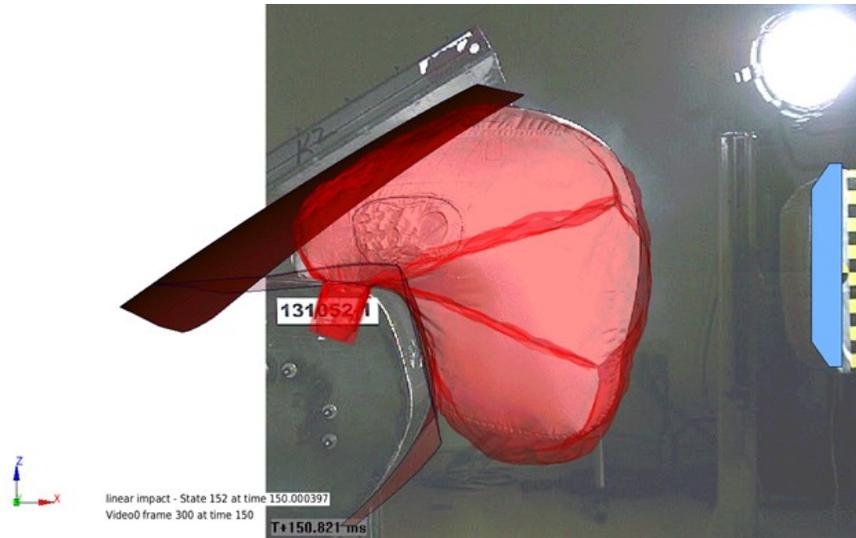
Figure 14. Good agreement with the test for the first stage deployment of a sealed vents airbag at 150 msec.
