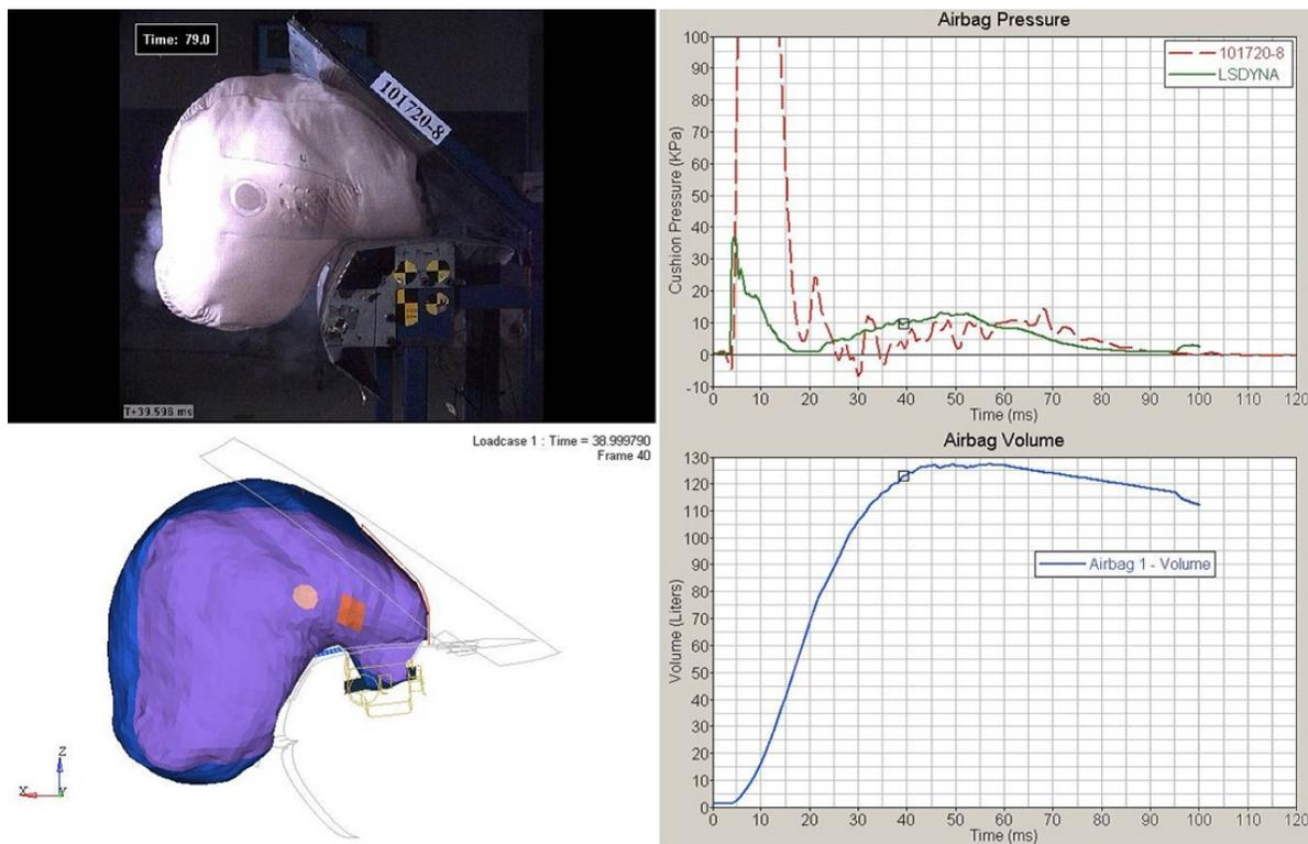
Figure 1. Dual stage static deployment correlation of the delivered PAB model.
