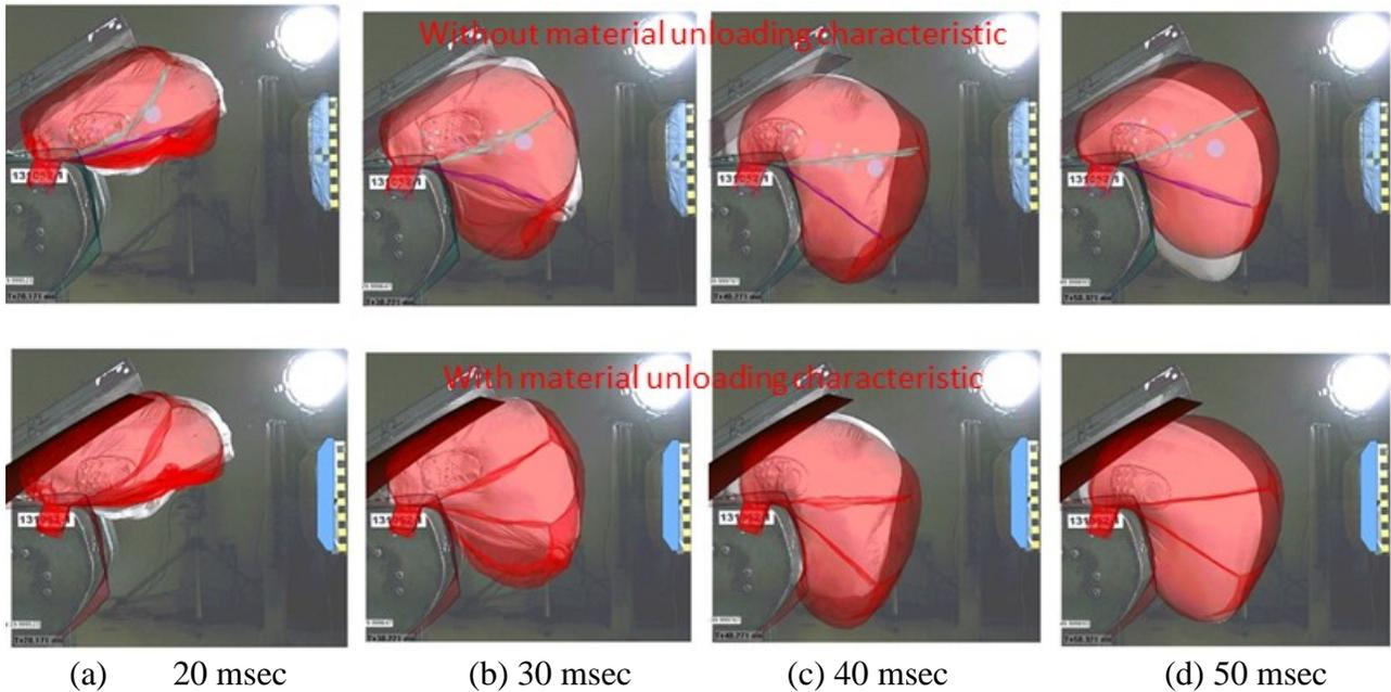
Figure 13. Comparison of the first stage deployment sequence of a vent-sealed airbag with (figure on the bottom) and without (figures on the top) modeling of the fabric material's unloading characteristic.
