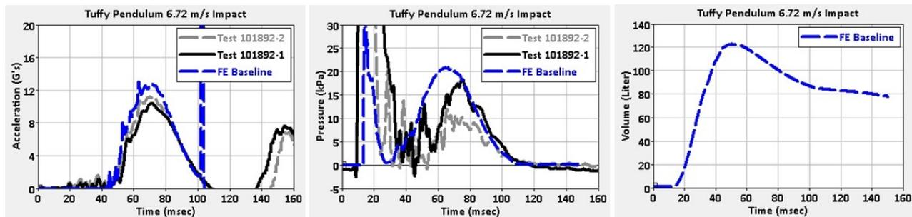
(a) Tuffy impactor deceleration (b) Airbag internal pressure (c) Airbag volume
