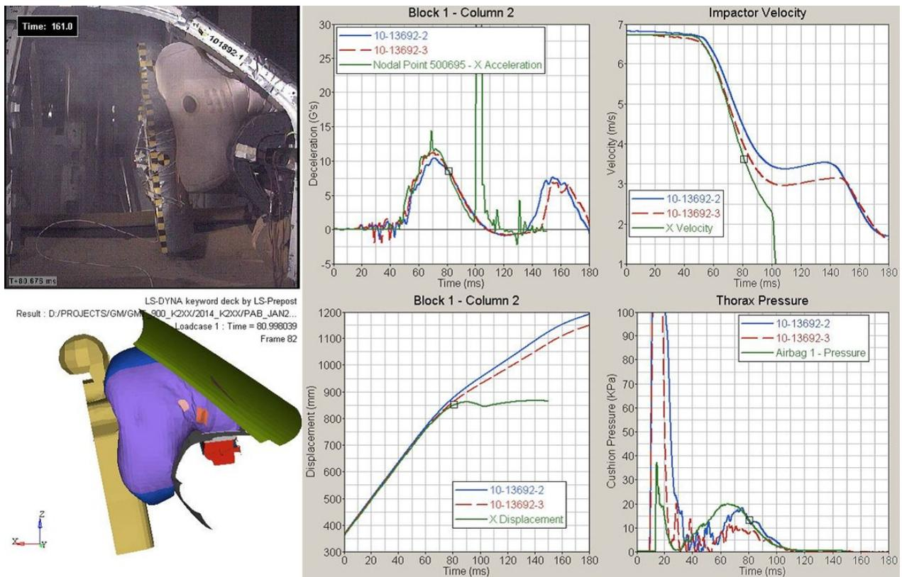
Figure 3. Thirty four kilogram Tuffy model impacting PAB with a higher velocity of 6.72m/s.
