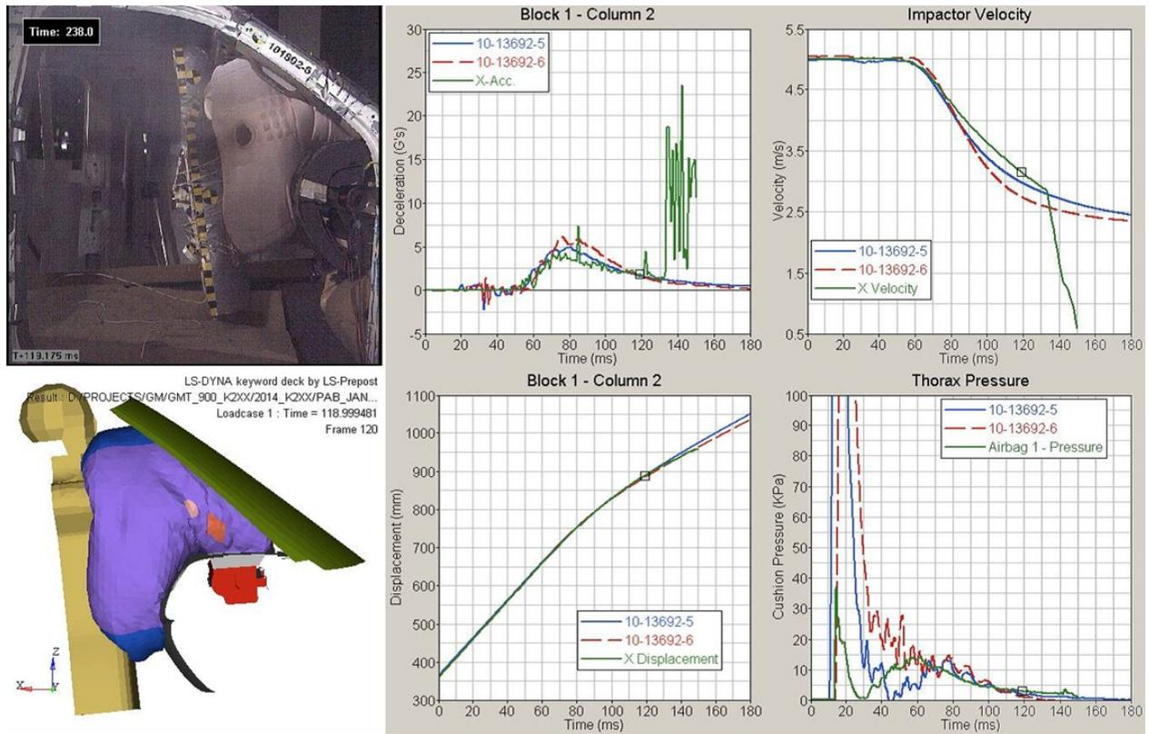
Figure 2. Thirty four kilogram Tuffy model impacting PAB with a velocity of 5.0m/s.
