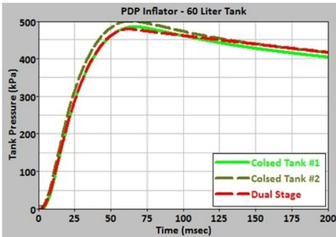
(a) Closed tank test for dual stage
