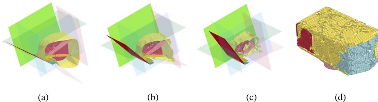
Figure 11. (a) Airbag enclosed by the plates before squashing, (b) in the midst of squashing, (c) further into the squashing process, (d) squashed and compressed airbag.
